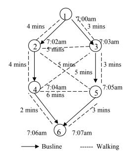
Figure 2 Representation of a Transportation Network
