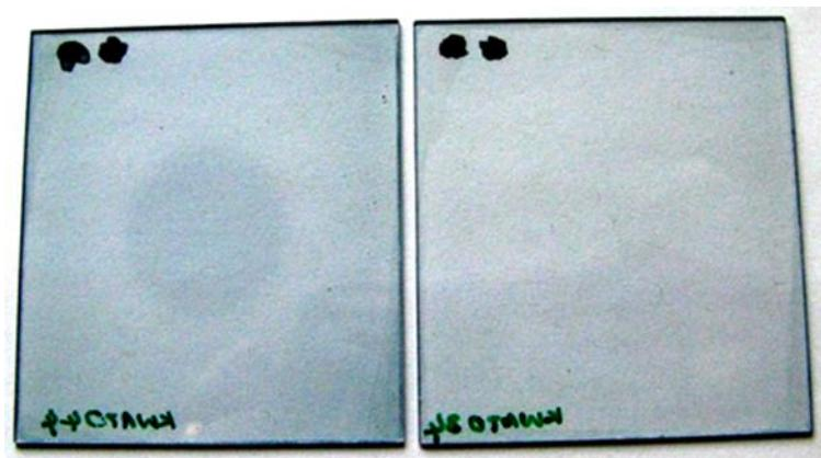
Figure 5.2: Spin coated  $\text{SnO}_2:\text{Sb}$  layers on Eagle XG glass substrate : left-12 spun layers right- 6 spun layers.
