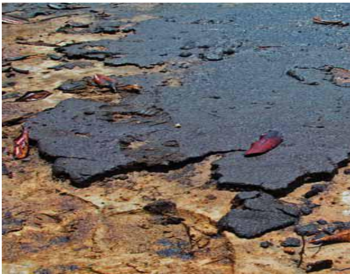
Fig 8.1: SOIL CAKED INTO CRUSTS OF DRIED CRUDE OIL
