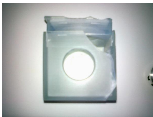
Figure 4.44 Breakage of the lighting unit casing because of tight tolerances in the joints.
