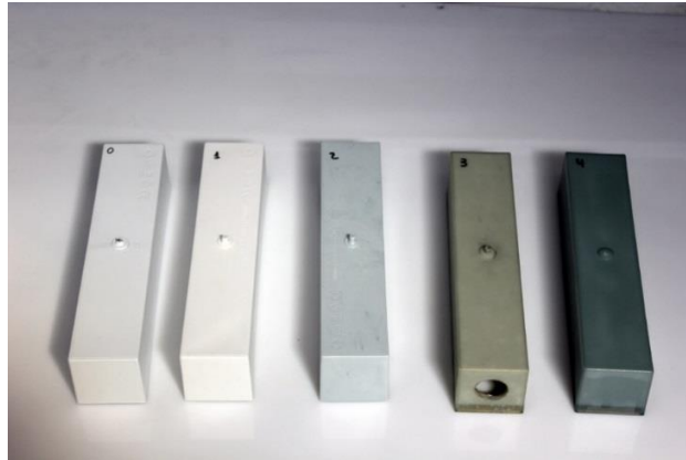
Figure 4.47. Housing-additives gradation: Housing with no additives (right housing) to maximum addition of additives (left housing)
