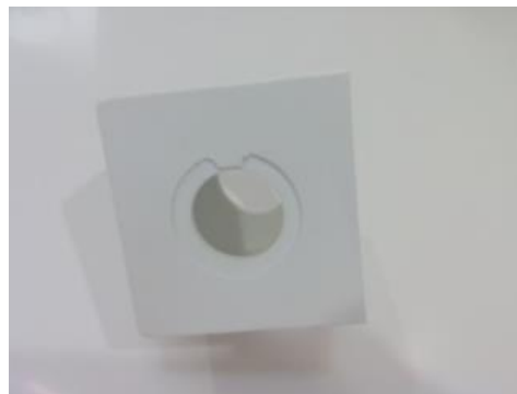
Figure 4.46. Design feature in the hole of the housing for the new joint-connector.
