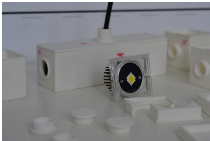
Figure 4.32. Prototypes made of nylon and detail of LED units with heat sink using transparent holders.
