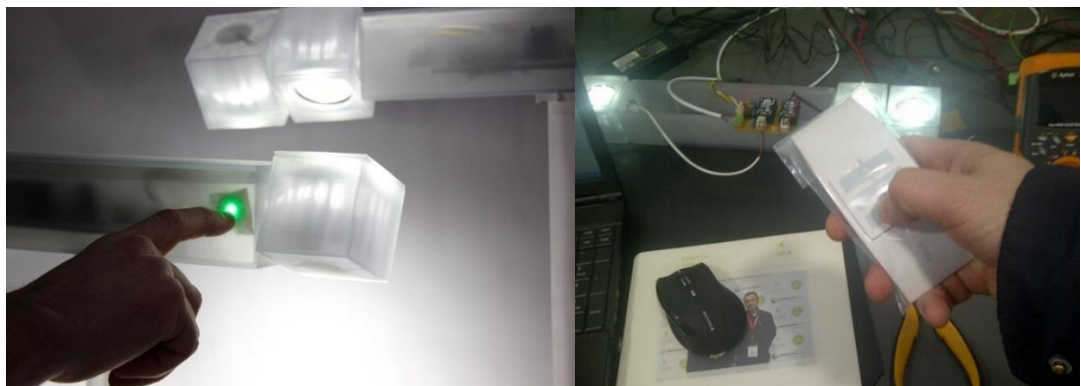
Figure 4.52. Touch-based switch controls built into the housing (left image). Wireless remote control testing (right image).
