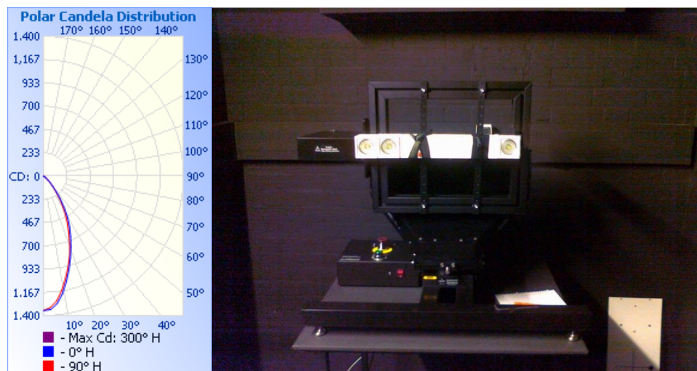
Figure 4.59. Light intensity distribution polar diagram of the lighting product (left image). Lighting product with three lighting modules mounted on the goniometer (right image).
