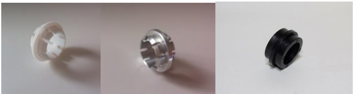
Figure 4.45. Snap-fit joint connector made of Teflon (left image). Snap-fit joint connector made of aluminium (centre image). Snap-fit joint connector made of recycled PET (right image).
