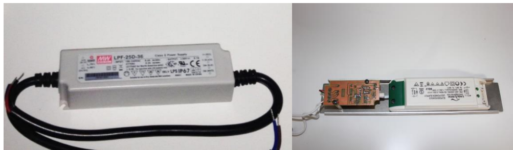
Figure 4.49. Initial driver selected (left image). Final driver selected with circuit integrated (right image).
