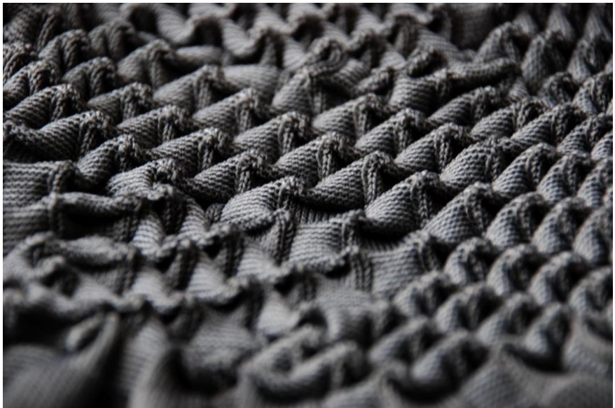
Figure 7.69 Sample 17 (Rectangle purl) Regular pattern plated with elastic, giving an irregular appearance.
