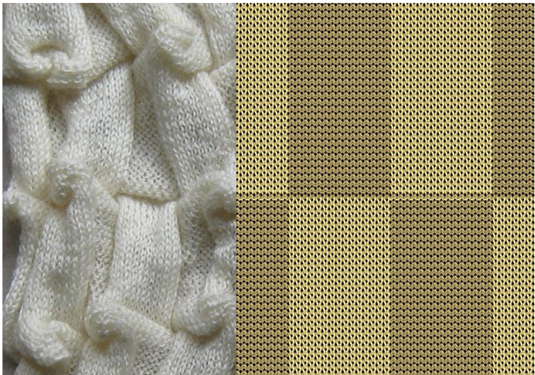
Figure 2.17 Photograph of Sample 4, 'Purl Rectangle' fabric ( Chapter 4: Stage I ) compared with image taken from Stoll MIplus software in 'fabric view'
