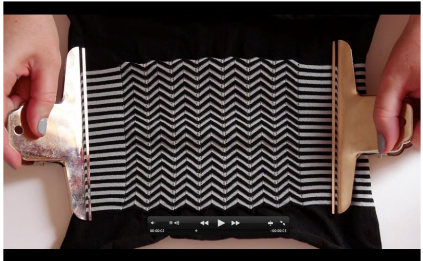
Figure 7.77 Sample 22 (TP4) knitted in grey and black covered elastic yarn at rest (a) and stretched in X-axis (b).
