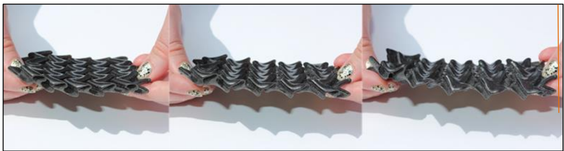
Figure 8.104 3D-print 2 showing expansion in the Z-axis when stretched.
