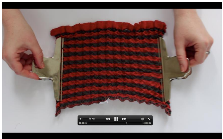
Figure 7.68 Sample 16 (Purl zigzag stagger) in stripes of grey and orange polyester at rest (a) and stretched in Y-axis (b).
