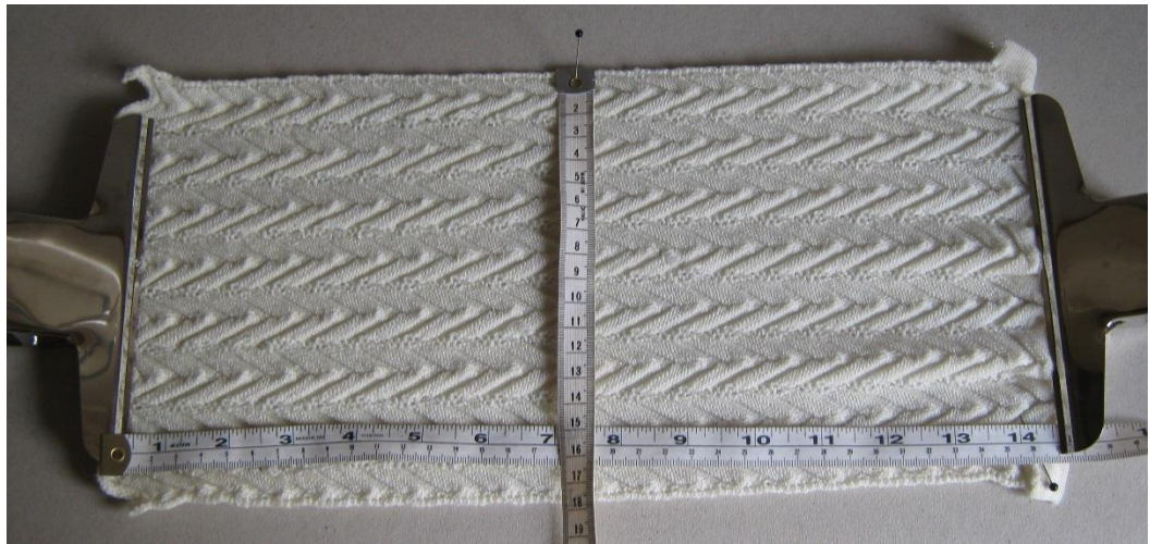
Figure 3.38 Photograph showing preliminary testing set up. This fabric is being stretched along the Y-axis.
