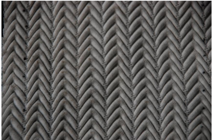
Figure 7.73 Sample 20 (TP4) knitted in 3 ends of Zimmerman elastomeric yarn.
