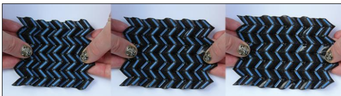
Figure 8.102 3D-print 1 showing auxetic behaviour when stretched (stretch occurs in the Y-axis and expansion in the X-axis when given comparative axes to the knitted fabrics in this study).
