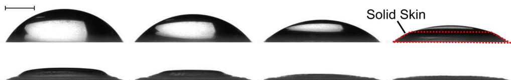
Figure 7.17: Time-lapse profile images of high molecular weight ( $M_W = 300$  kg/mol) droplet under reduced pressure ( $P = 500$  mbar) showing an apparent growth of solid skin up the surface of the droplet, rather than the previously observed receding contact line stage. Scale bar represents 1 mm.
