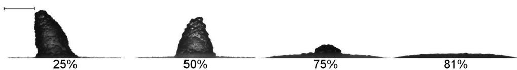
Figure 6.9: Fully dried profile images of droplets dried in the relative humidity range 25-80%.  $c_0 = 10\%$ .
