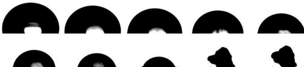
Figure 5.27: Profile images of a  $c_0 = 5\%$ ,  $V_0 = 10 \mu\text{l}$  droplet on a Cytop coated substrate. No pinned stage observed, rather the droplet freely recedes until it precipitates uniformly leading to large central solid clump. Images courtesy of Manon Granjard from the University of Edinburgh.
