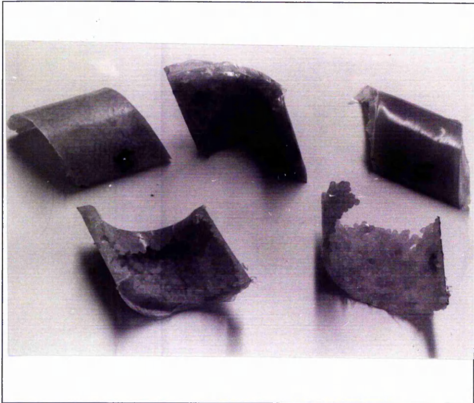
Figure 4.6 Material cuttings, stripped off the screw.
