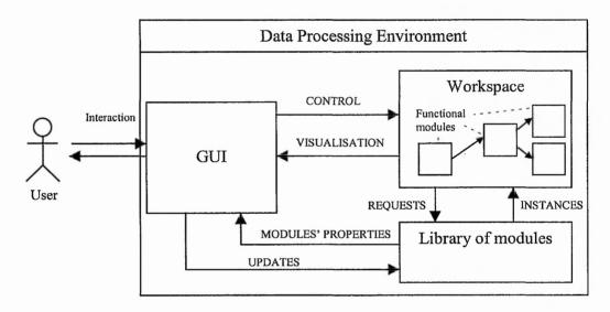
Figure 4.10. The system's architecture
