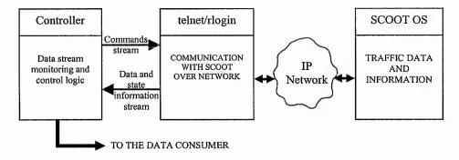
Figure 3.7. Architecture of data acquisition procedure
