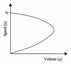
Figure 2.2. Typical speed-flow curve
