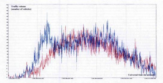
Figure 6.5. Example of traffic profiling module output visualised by Plot module. Data used is taken for the N60411M1 detector for 16<sup>th</sup> January 1999, Saturday (red) and 19<sup>th</sup> January 1999, Tuesday (blue) and aggregated over 2 minutes intervals.
