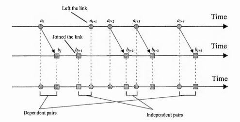
Figure 5.6. Illustration of the concept of dependent and independent pairs
