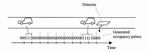
Figure 3.3. SCOOT detector data flow
