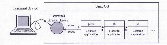
Figure 3.5. Hierarchy of applications and forwarding of the terminal IO streams
