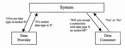
Figure 4.9. Illustration of the data typing system
