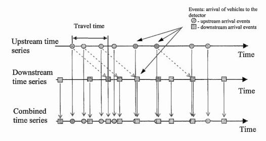
Figure 5.3. Merging upstream and shifted downstream time series
