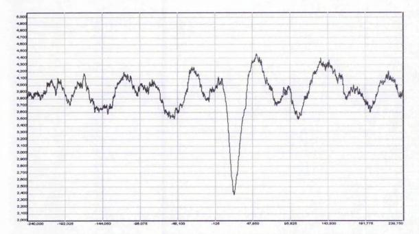
Figure 6.13. Cost function of link N60331F1-N60421B1 in a bigger scale. Several minimums point to the similarities due to cyclic nature of the series. The global minimum points to the "best match" between the series. Time shift varies from -4 minutes to 4 minutes. The global minimum is reached at time shift equal 24.25 seconds.
