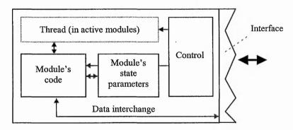
Figure 4.8. Structure of a module wrapper
