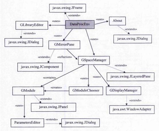
Figure 4.11. GUI classes architecture
