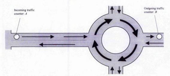
Figure 5.9. The link model: a roundabout between two measuring points *A* and *B* allows vehicles to leave and join traffic flow
