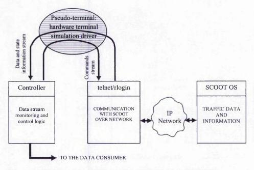
Figure 3.8. Architecture of data acquisition procedure with pseudo-terminals
