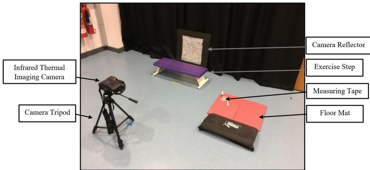
**Figure 3.4.** Equipment used for conducting the infrared thermal imaging on participants; including the infrared thermal imaging camera, tripod, exercise step (used for participants to stand on during image capture), floor mat (used to limit participant contact with cold floor), tape measure (used to define landmarks), and camera reflector (used to measure reflected temperature).
