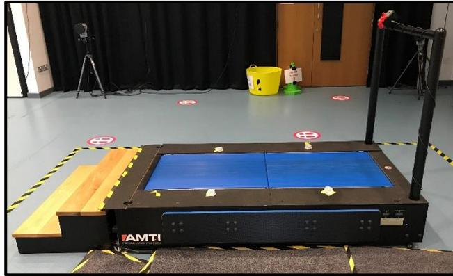
**Figure 3.8.** AMTI instrumented treadmill, used in Chapter 9, which comprises of two separate treadmill belts with a force platform located under each belt.
