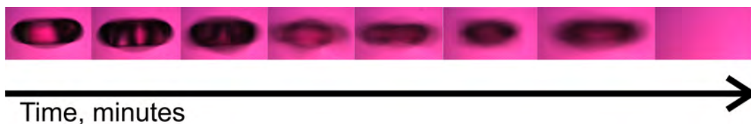
Figure 3.10: A time series showing an example of the droplet oscillation which causes the droplet to fall from the trap when levitated in the TinyLev acoustic levitator.
