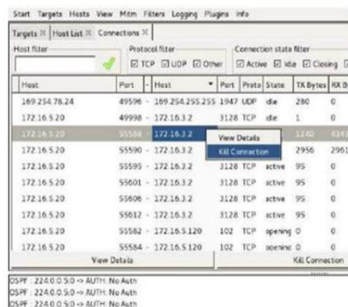
Figure 4. Killing target connections using Ettercap
