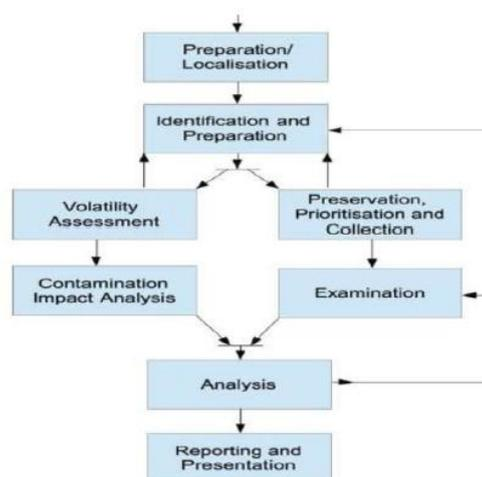
Figure 1. SCADA Incident Response and Forensic Process
