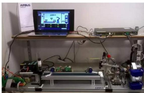
Figure 2. SCADA Production Line Testbed
