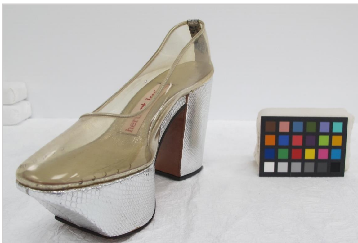
Figure 44. Polyvinyl chloride evening shoes showing yellow discolouration due to PVC degradation. Beth Levine, manufactured by Herbert Levine Inc., c.1970. Brooklyn Museum Costume Collection at The Metropolitan Museum of Art, Gift of the Brooklyn Museum, 2009; Gift of Beth Levine, 1996 (2009.300.6110). Image: ©Leanne Tonkin. The Metropolitan Museum of Art, 2016.
