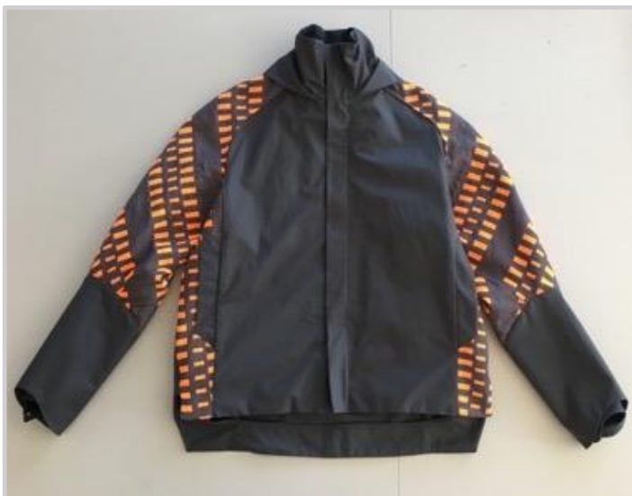
Figure 62. Woven cycling jacket incorporating LEDs within electronic yarns in the elbow, Nottingham Trent University, 2019. Image: ©Leanne Tonkin. Nottingham. 2020.
