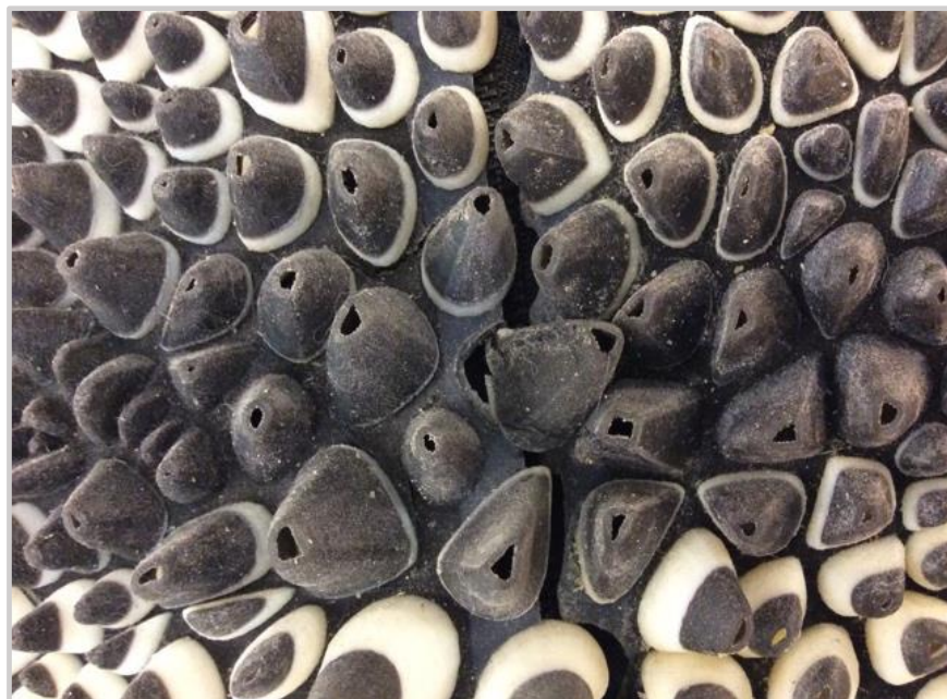
Figure 52. Breakage, discolouration and surface debris. Anthozoa 3D skirt, Voltage Collection 2013, designed by Iris van Herpen, Neri Oxman and Julia Koerner in collaboration with Stratasys. Museum of Fine Arts, Boston. c.2013. (2013.1487.1). Image: ©Leanne Tonkin. 2017.
