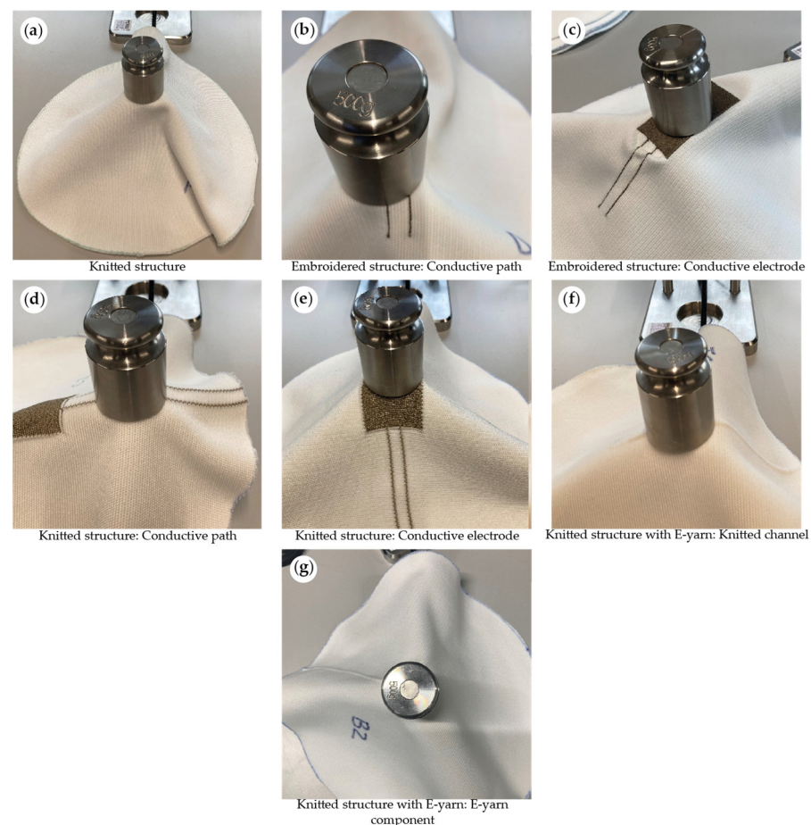
Figure 4. Images of the samples placed on the C-Therm. This shows the exact locations that were tested. (a) Locations tested on knitted structure samples. (b,c) Locations tested on embroidered electrode samples. (d,e) Locations tested on knitted electrode samples. (f,g) Locations tested on knitted structure with E-yarn samples.
