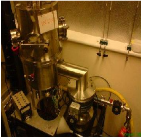
Figure 3.10 - Left – Photograph of evaporation system. Right – Schematic of evaporation system
