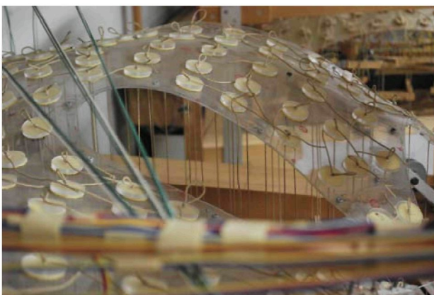
Figure 2: Detail of experimental model for design of the shell at Sicli, Geneva – Isler office, 2011 (Photo: John Chilton)
