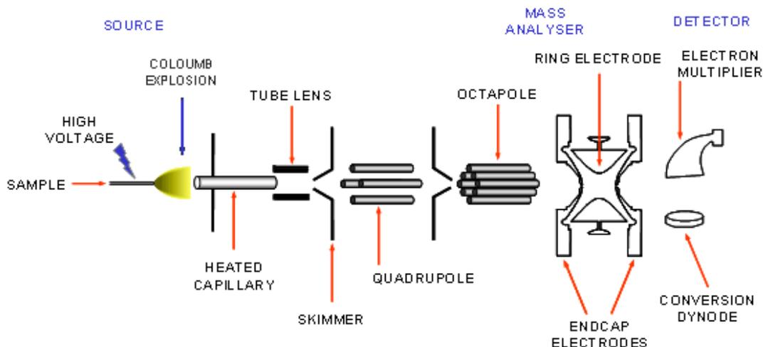
**Figure 6.1:** Schematic design of a Fisher Thermo LTQ ESI MS/MS (adapted from Fisher online).
