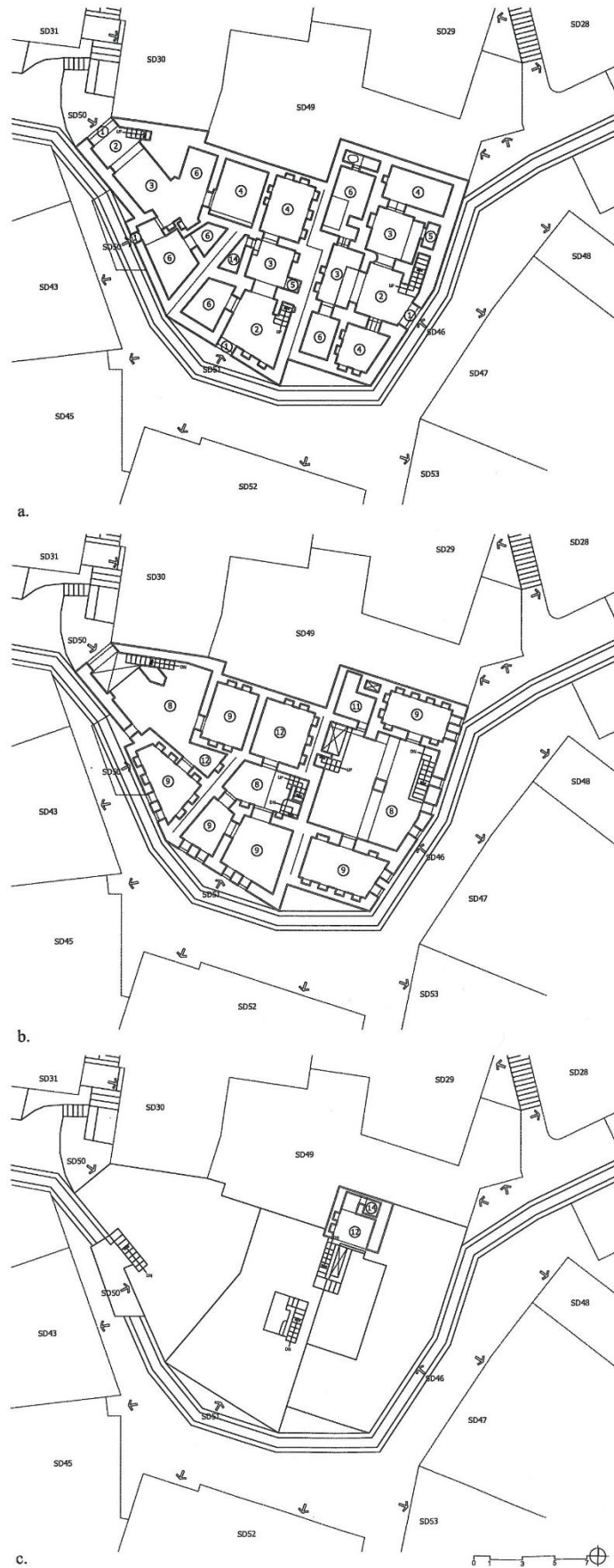
Plate 28: Floor plans of dwelling cluster SD46, SD50 & SD51; a. Ground floor; b. First floor; c. Roof and second floor; 1. main entrance door; 2. First dahreez ; 3. Second dahreez ; 4. suffah ; 5. ‘aqid ; 6. darss ; 8. ‘arshah ; 9. gurafah ; 11. Kitchen store; 12. Kitchen; 14. Latrine.
