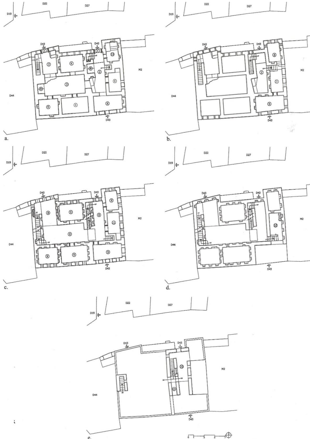
Plate 33: Floor plans of dwelling SD43; a. Ground floor; b. First mezzanine floor; c. First floor; d. Second mezzanine floor; e. Third floor and roof; 1. main entrance door; 2. First dahrīz ; 3. Second dahrīz ; 4. suffāh ; 5. ‘aqad ; 6. darss ; 8. ‘arshah ; 9. guraḥ ; 10. Overhead shade; 11. Kitchen store; 12. Kitchen; 13. Falaj bath; 16. Sky light.
