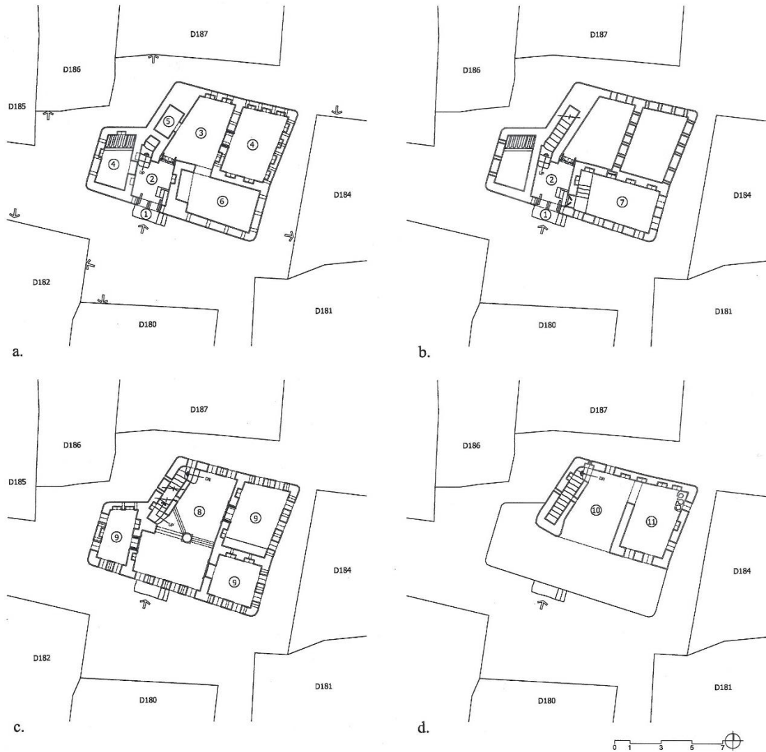
Plate 21: Floor plan of D183; a. Ground floor; b. Mezzanine level; c. First floor; d. Roof and second floor; 1. main entrance door; 2. First dahreez ; 3. Second dahreez ; 4. suffah ; 5. ‘aqid ; 6. darss ; 6. sblah ; 7. sblah ; 8. ‘arshah ; 9. guraḥah ; 10. shade; 11. Kitchen.
