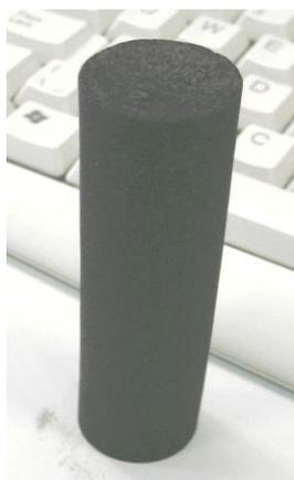
**Fig.V.2:** Photograph of an AC composite cylindrical sample. The actual height of this cylinder is 7 cm and its diameter is 2.4 cm.
