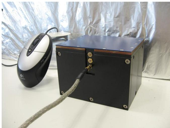
**Fig.II.4:** Photograph of the *profile* NMR Mouse<sup>®</sup> connected to the RF transceiver (not shown), easily transportable due to its light weight (5.2 kg) and moderate size. A PC mouse on the left is also shown to give an idea of the actual size of the NMR Mouse<sup>®</sup>.
