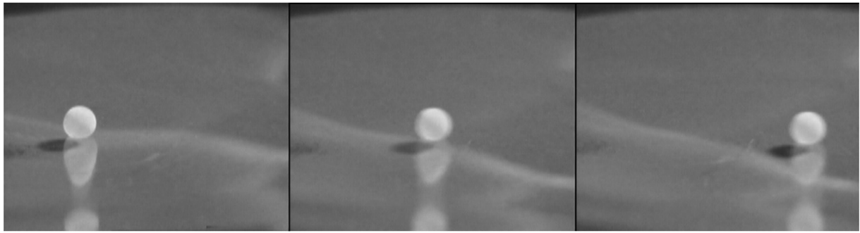
Fig. 21. A liquid marble of water with hydrophobised lycopodium powder rolling across a Petri dish.
