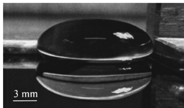
Fig. 20. Leidenfrost drop; water on a heated surface, Reproduced with permission from Bianco et al. [87]. Copyright American Institute of Physics.
