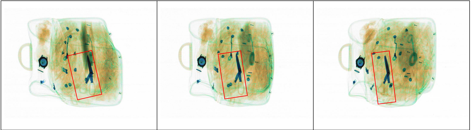
Bag 3: Large scissors with plastic handles no mask and maximum footprint, in the centre of a small soft case bag.
