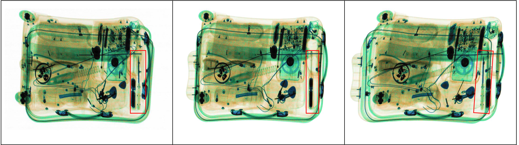
Bag 14: Medium size kitchen knife masked by an electric toothbrush, at the periphery of a wheeled bag.
