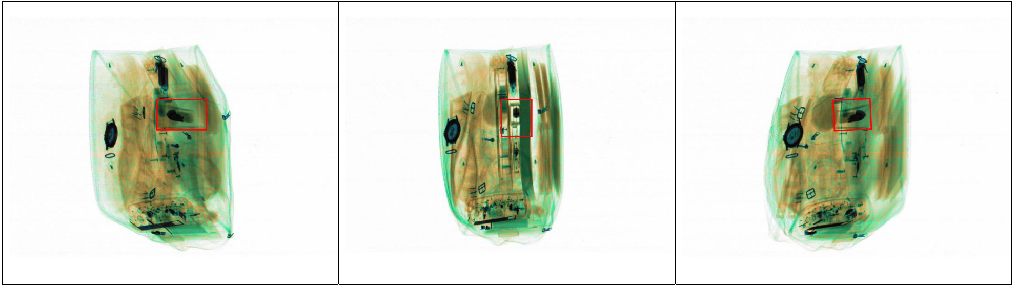
Bag 16: Small size kitchen knife (ceramic) at a minimum footprint with no mask, in the periphery of a small soft case bag.
