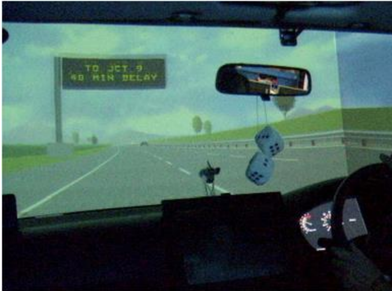
Fig. 1 Driving simulator displaying VMS
