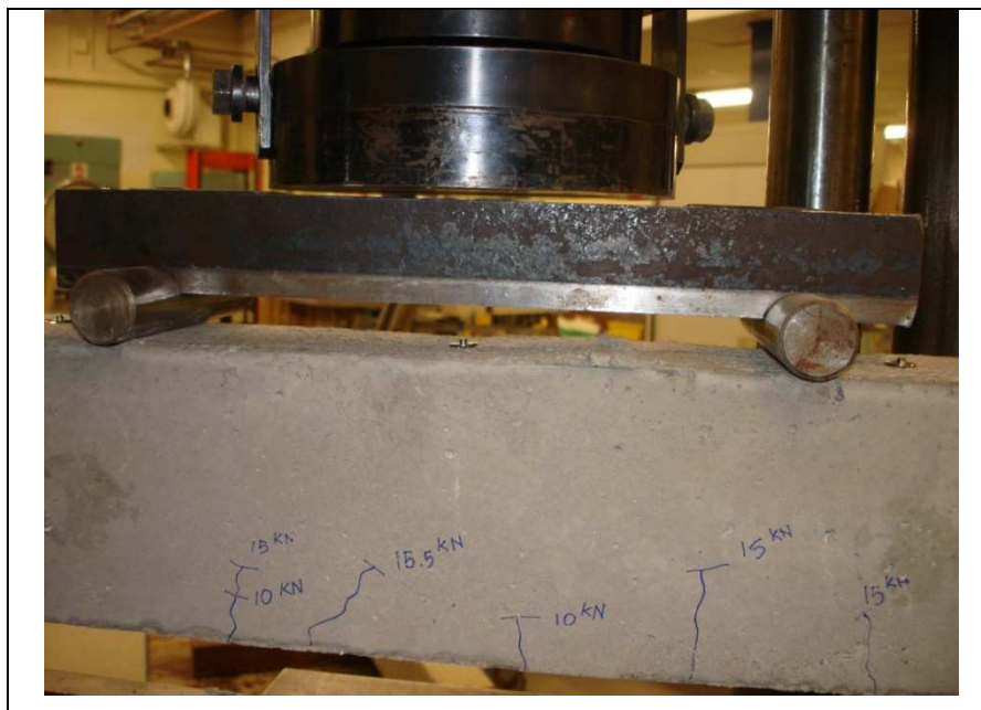
Figure 6.4: Beam B - mid span zone at the final damage state- photograph.
