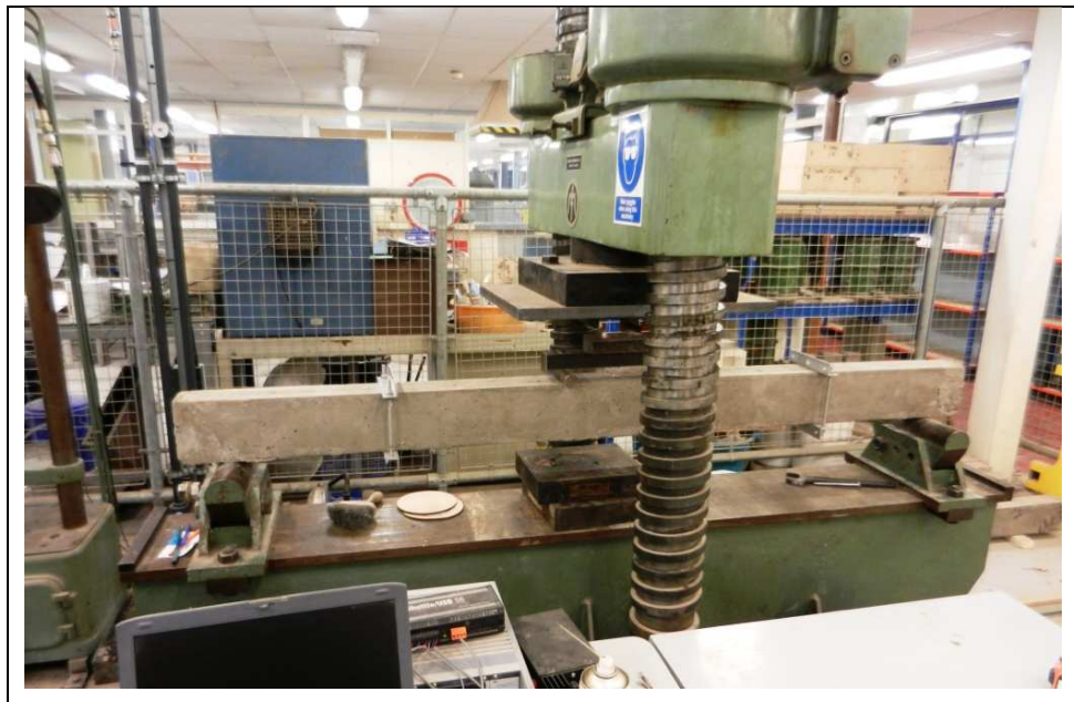
Figure 6.6: Beam C - under one of the static loading stages- photograph.
