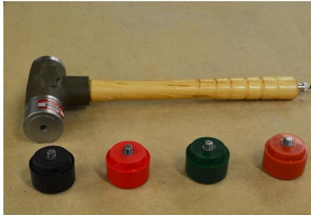
**Figure 4.5:** Delta Tron version 8208 instrumented impact hammer with four tips.
