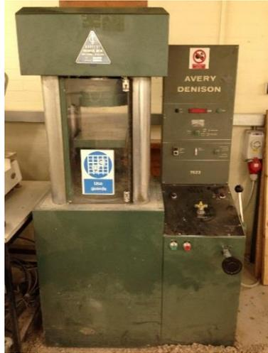
**Figure A. 9:** Concrete compression testing machine.
