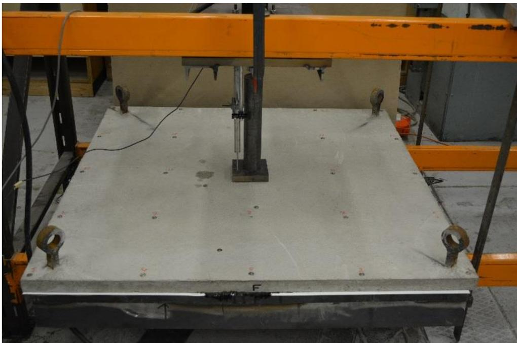
**Figure A. 16:** Placement the partially concentrated load on slab centre.
