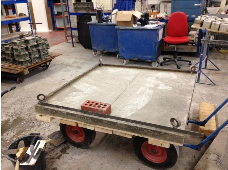
**Figure A. 5:** Create a water pond over the RC slab surface for its curing.
