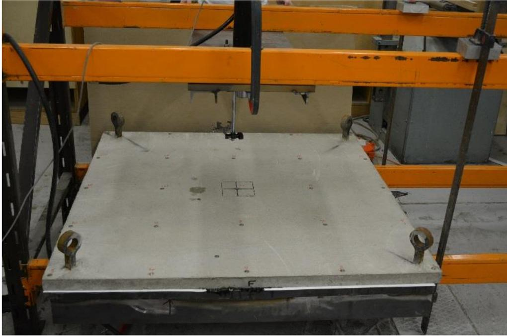
**Figure A. 15:** Marking the location of partially concentrated load on slab centre.
