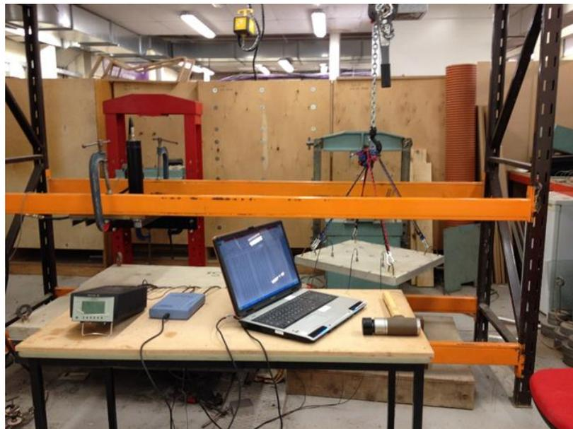
**Figure 4.24:** Test slab (600x600x40mm) under free-free boundary condition.
