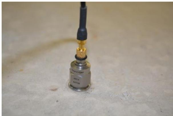
**Figure 4.7:** Delta Tron® model 4514 accelerometer.
