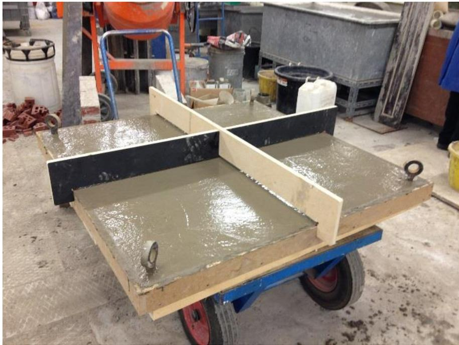
**Figure A. 4:** Completion the concrete slab casting process.
