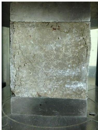
**Figure A. 11:** Concrete cube failure under compression testing machine.
