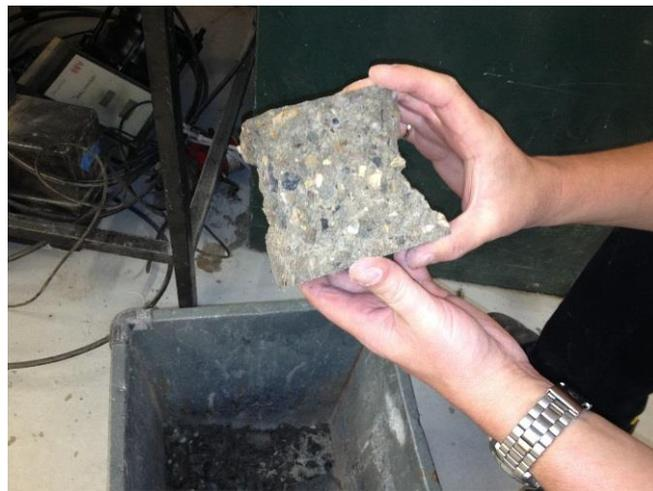
**Figure A. 13:** Final shape of failed concrete cube.
