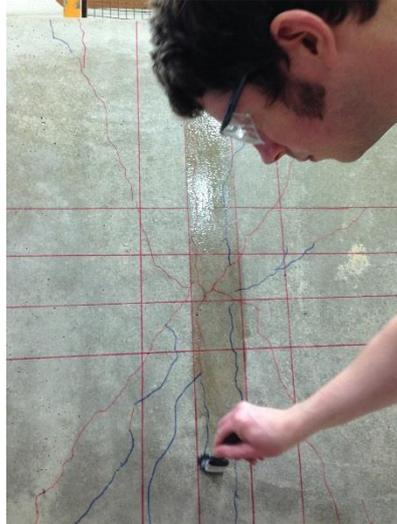
**Figure A. 21:** Coating the epoxy adhesive to the marked locations on the tension surface.
