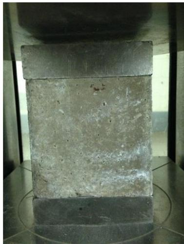
**Figure A. 10:** Confinement of a concrete cube.
