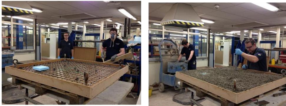
**Figure 4.28:** Artificial void induced on the surface of the slab during the casting process.
