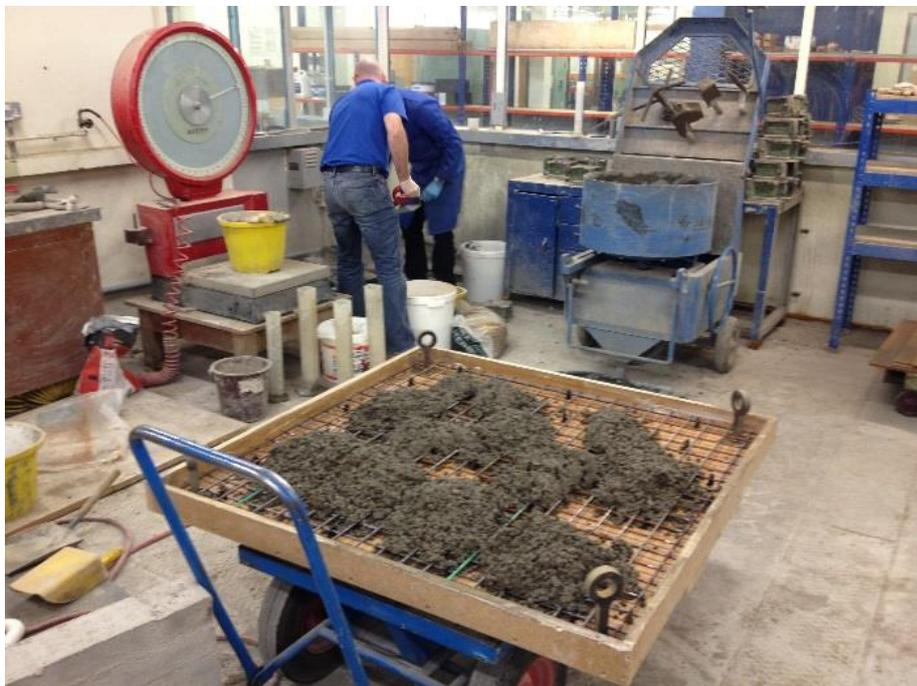
**Figure A. 3:** Placement of some concrete batches into the well-oiled mould.
