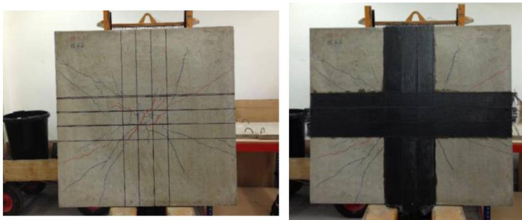
**Figure 4.27:** Strengthening RC slab with CFRP sheet.
