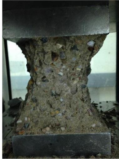
**Figure A. 12:** Continuous failure to concrete cube.
