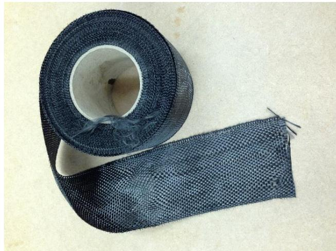
**Figure A. 19:** CFRP fabric roll.
