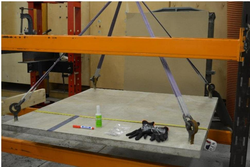
**Figure A. 14:** Preparation the equipment to mark the slab with a grid of response points.
