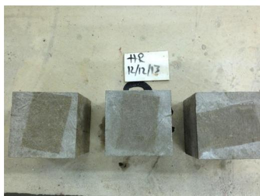
**Figure A. 8:** Removing the concrete cubes from the curing water basin and preparing them for testing
