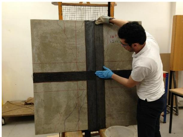
**Figure A. 23:** Continuous process of Strengthening RC slab specimen with CFRP sheets.
