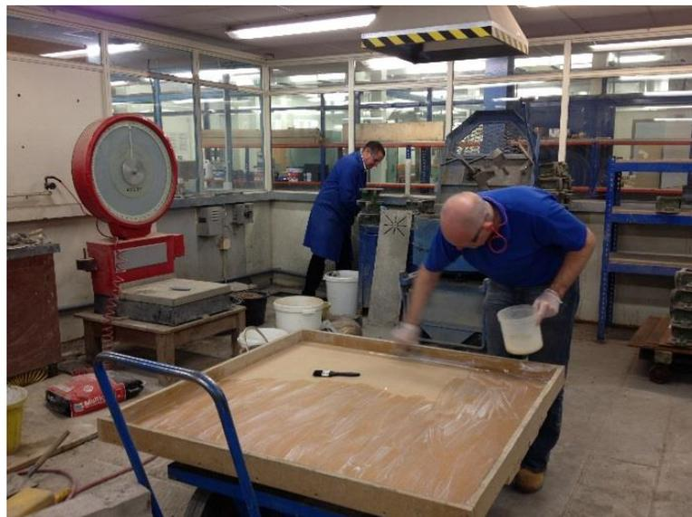
**Figure A. 1:** Oiling the mould with release mould agent before being ready for use.
