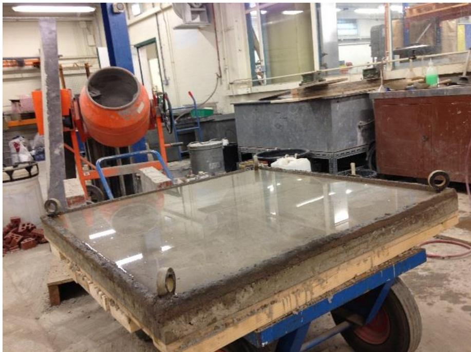
**Figure A. 6:** A reinforced concrete slab ponded while curing in the laboratory.
