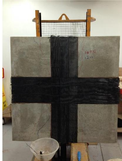
**Figure A. 24:** View of RC slab after completion of strengthening with CFRP sheets.
