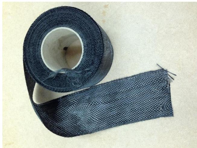
**Figure A. 19:** CFRP fabric roll.
