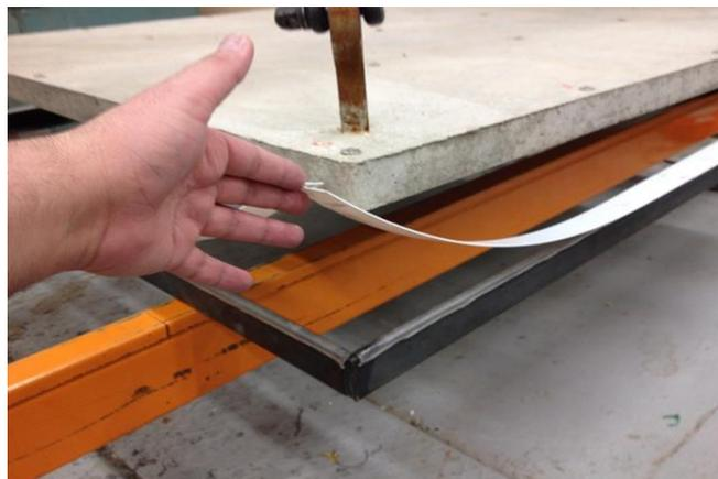
**Figure 4.25:** Rubber pipe and HIPs been placed onto the support contact line.
