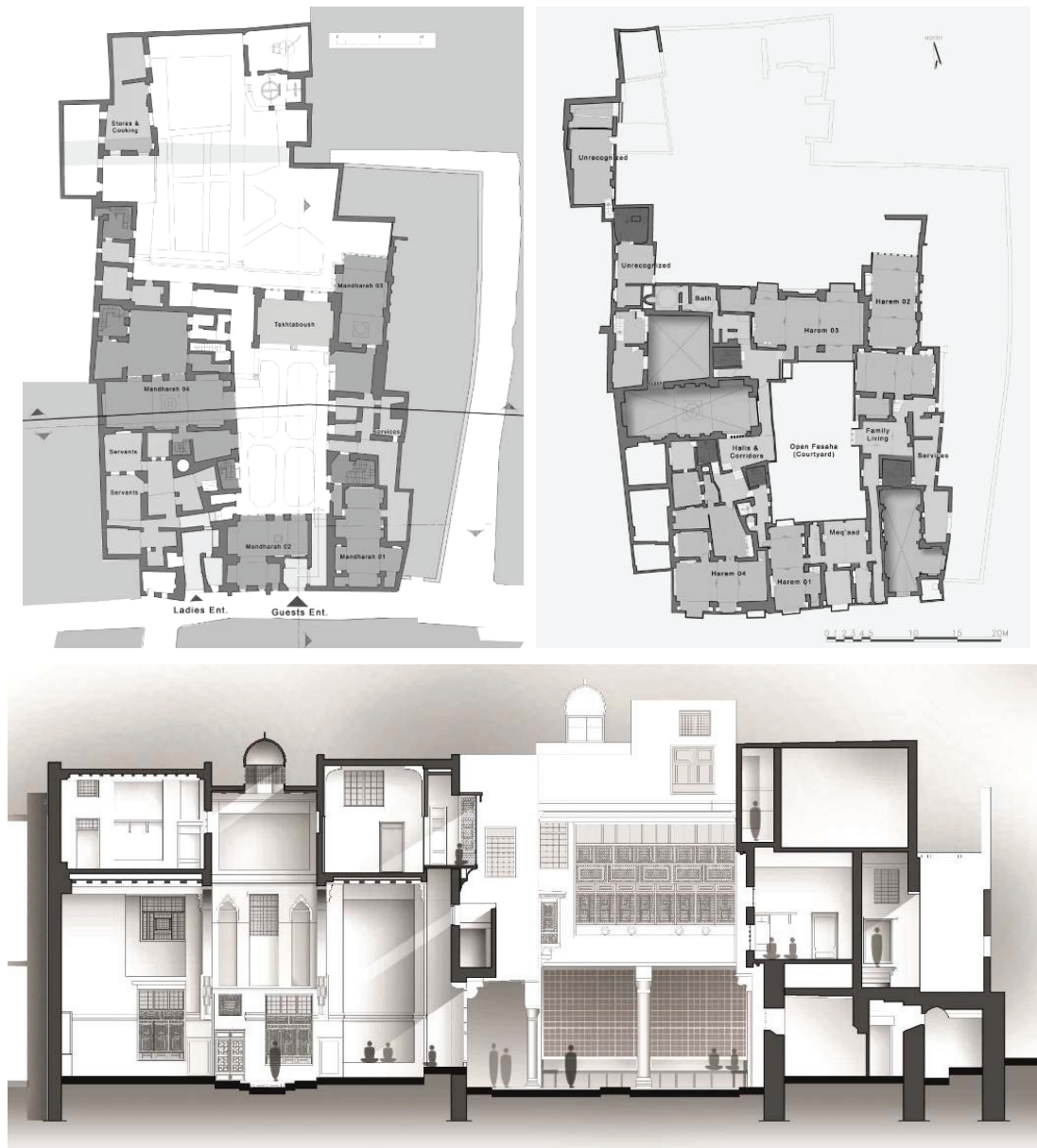
Fig. 5 Bayt al-Suhamiy's Floor plans and a section showing the ground floor public sphere.
