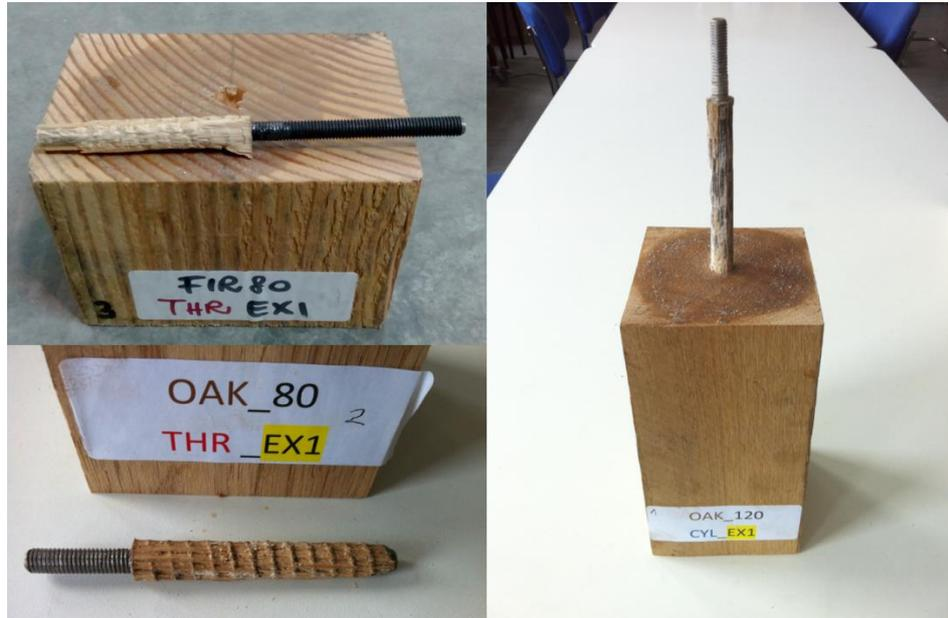
*Fig. 5-27: cylindrical and threaded samples of adhesive anchors of made by EX 1:1 (grey) after being tested by pull-compression tests in confined regime*
