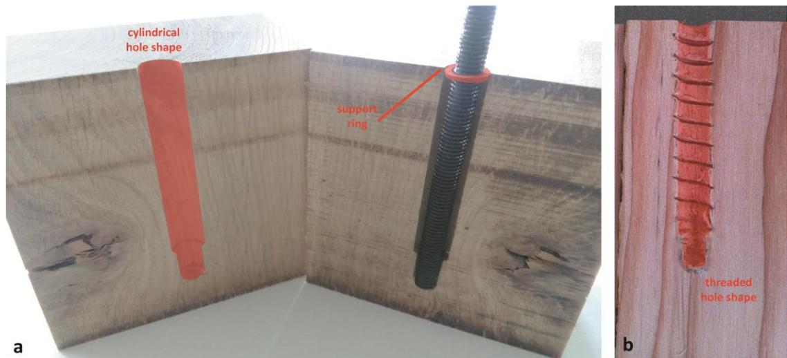
Fig. 6-7: sample characterised by a cylindrical hole shape (a: left) and by a threaded hole shape (b: right)
