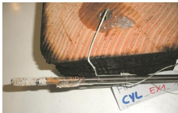
*Fig. 6-13: thermal degradation of the external part of the embedded steel rod as a consequence of a severe heating process*
