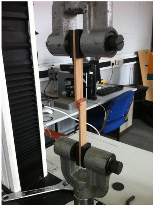
*Fig. 4-9: tensile test on a single lap-joint*
