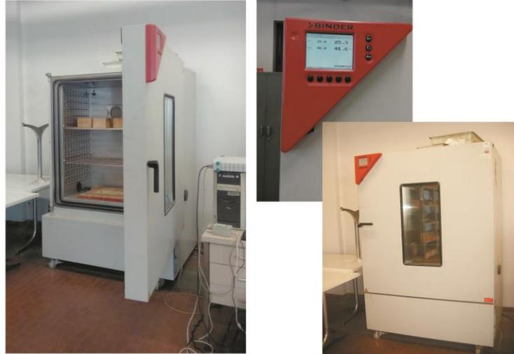
Fig. 6-5: BINDER climatic chamber used for samples conditioning
