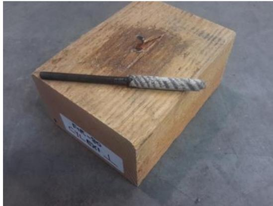
Fig. 5-31: tested sample of a resin connector made of an 8 mm steel bar glued perpendicular to the wood (solid Douglas Fir) grain in a cylindrical borehole
