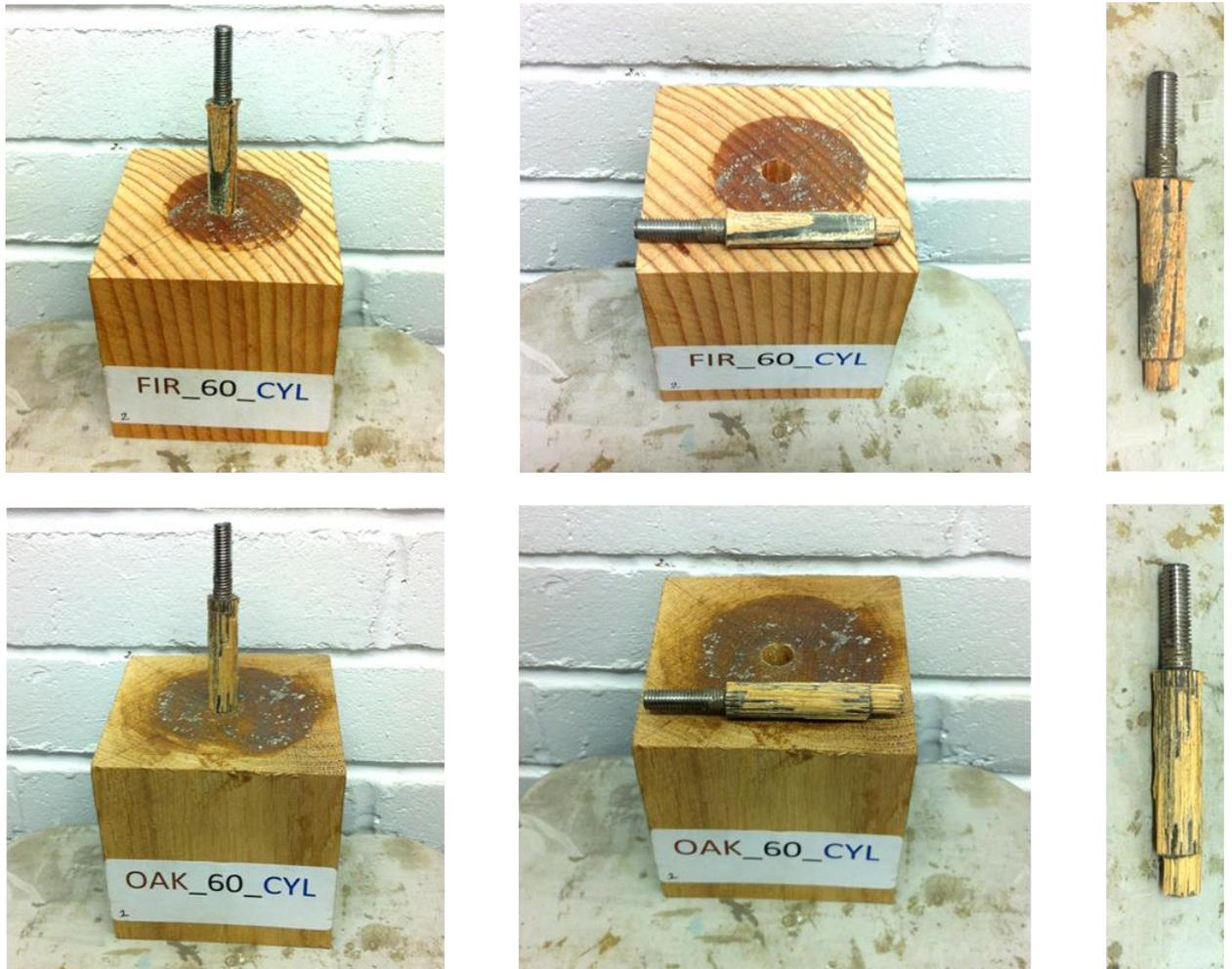
*Fig. 5-12: cylindrical (CYL) tested samples (Di Maria and Ianakiev 2015)*
