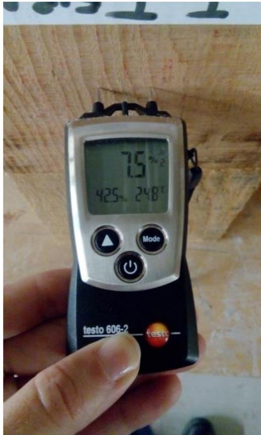
Fig. 1-4: TESTO 606-2 pin-moisture meter for timber and building materials
