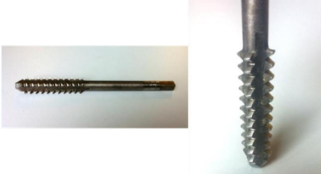
*Fig. 5-4: drill bit for woodworking (12 mm external diameter) (Di Maria and Ianakiev 2015)*
