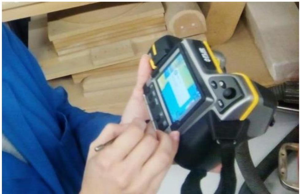
*Fig. 1-10: FLIR B200 thermal imaging camera*
