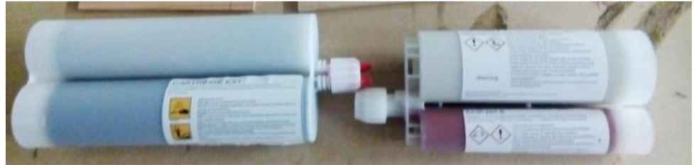
*Fig. 1-13: cartridges of epoxy resins: EX 1:1 (left) and EX 3:1 (right)*
