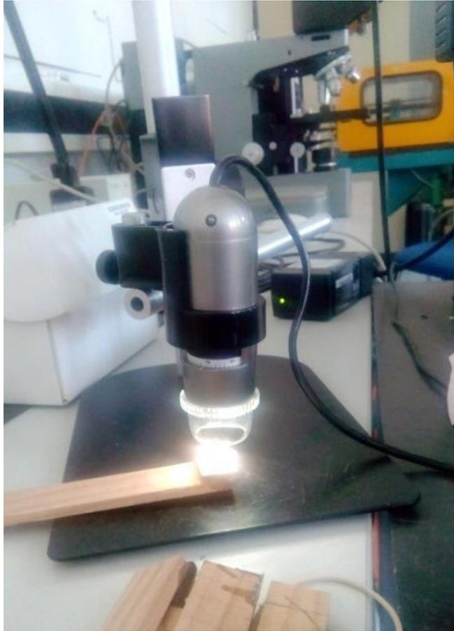
*Fig. 1-9: 300X usb-microscope*
