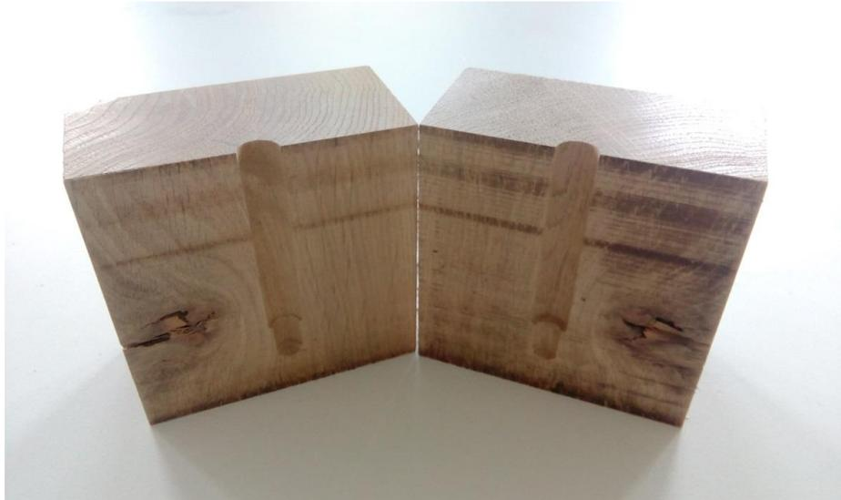
*Fig. 5-6: internal cylindrical and smooth surface in an Oak timber samples which presents a change in the size diameter at the bottom of the hole to solve bar's stability issues.*
