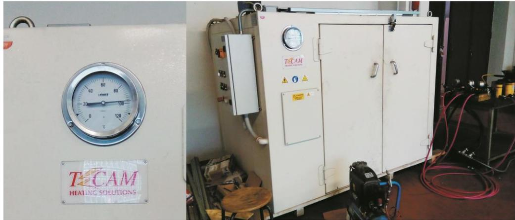
*Fig. 6-6: heating cabinet used to assess timber moisture contents*
