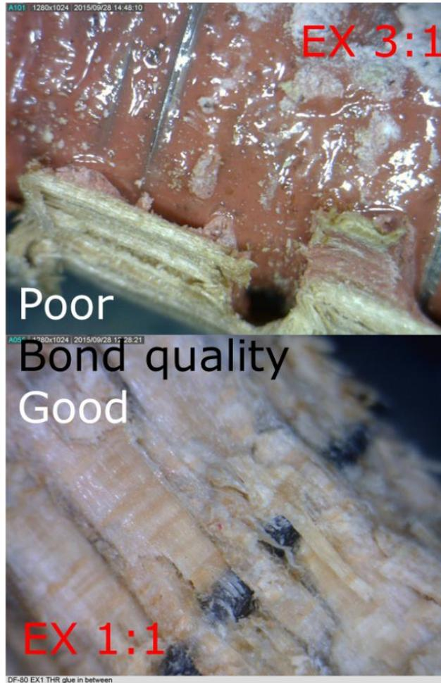
*Fig. 5-35: bond quality comparison by microscope images (50X magnification) of threaded samples of adhesive anchors in timber glued by high (EX 3:1: top) and low (EX 1:1: bottom) viscosity epoxy resins after being tested.*
