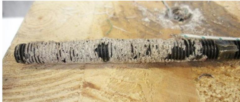
*Fig. 6-14: “crumbling effect” in the epoxy resin after being exposed to elevated temperatures*
