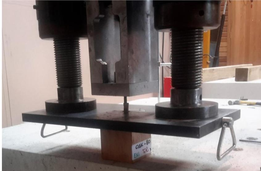
*Fig. 5-21: fatigue testing machine Dennison Mayer (load cell: 500 kN) located at the 2K polymer systems laboratories in Alfreton, UK*
