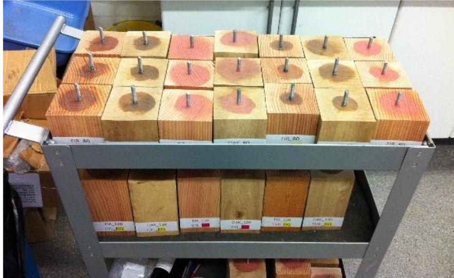
Fig. 5-16: test samples for experimental part 2 made of EX 1:1 and EX 3:1
