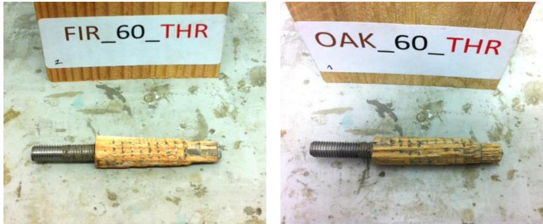
*Fig. 5-14: threaded hole shape samples made from Oak and Douglas Fir timber species (Di Maria and Ianakiev 2015)*
