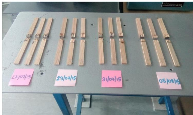
*Fig. 5-19: same samples of tested lap joints for tests about the shelf life of epoxy contained in a single cartridge*
