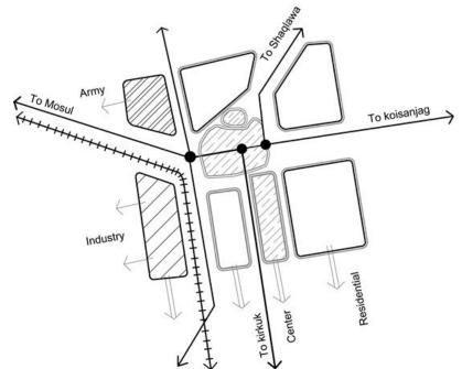
**Figure 5.15:** Doxiadis's sketch of the zonal function and main roads of Erbil **Source:** Modified and redrawn from (Doxiadis 1959, p. 11)
