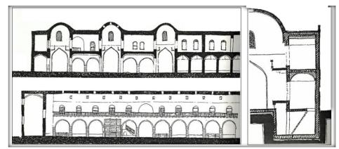
**Figure 7.8**: The section of one of the qaisarias **Source:** Modified from (Al-Dabbagh 1988, p. 80)
