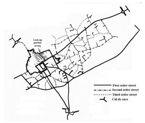
**Figure 1.19**: The routes gradation in the traditional city **Source:** Modified from (Hakim 2008, p. 66)
