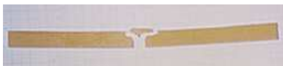
Figure 25 Failure and Tension break of typical sample.
