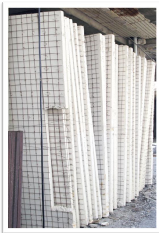
Photo 7: Foam sections for building walls
