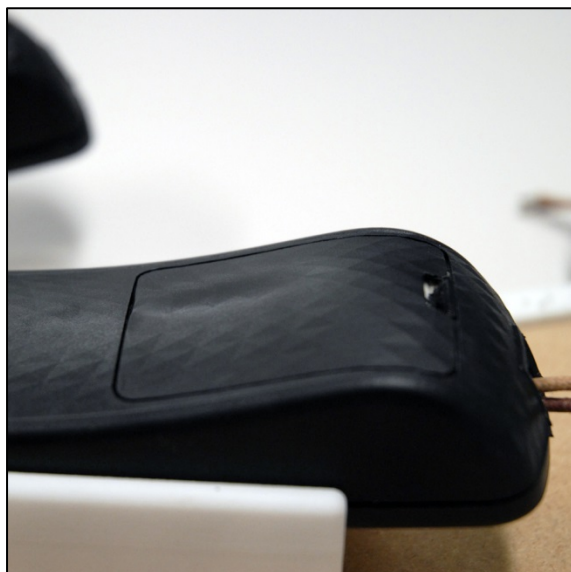
Fig.10 Sample with signs of heat damage
