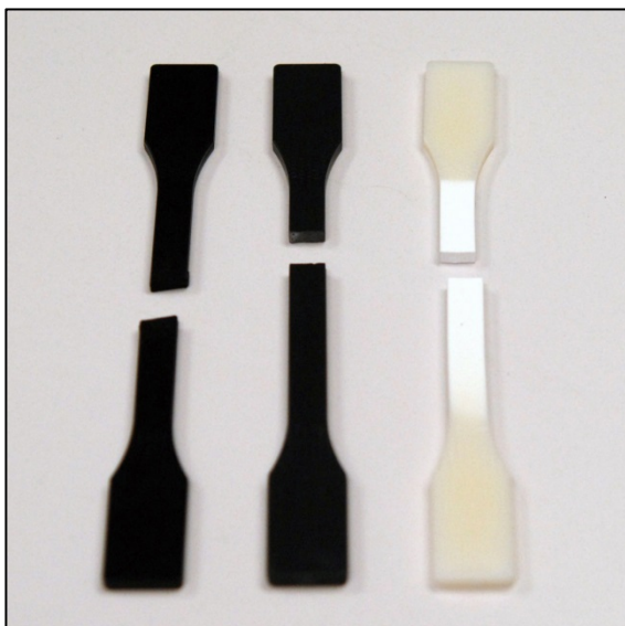
Fig.31 Material sample plaques post-test (left to right) rABS/PC, rABS, ABS
