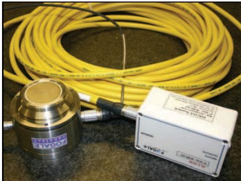
Figure 2: HLS sensor 4<sup>th</sup> generation with remote electronic, temperature sensor and cable
