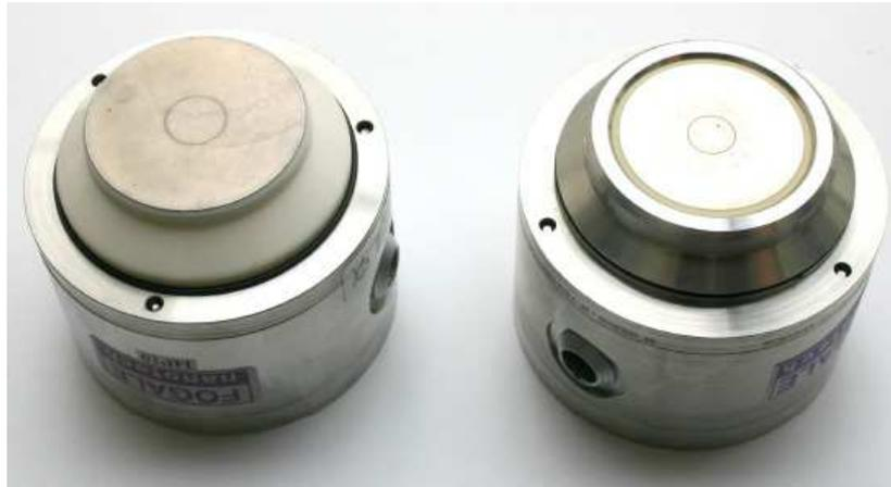
**Figure 1.** Two different types of HLS sensors (left: 1<sup>st</sup> generation, right: 4<sup>th</sup> generation)
