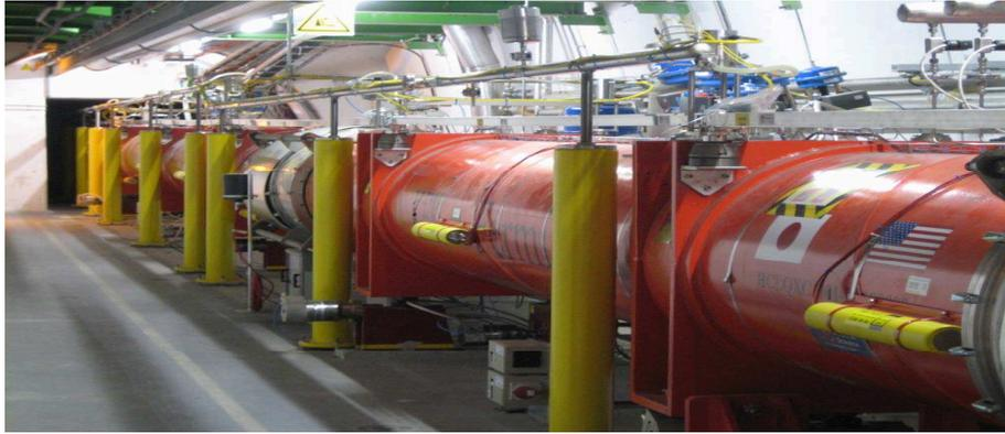
Figure 1.3: low-beta magnets in the LHC tunnel
