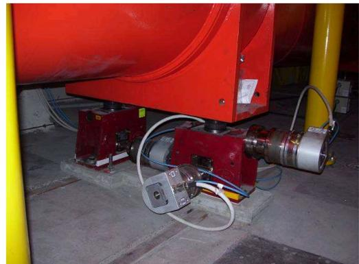
Fig. 4: Motor assemblies plugged on jacks
