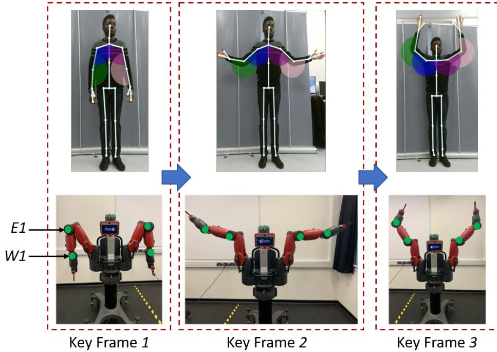
Figure 6.10: Final motions of Baxter assistive robot from the transferred human activity information.
