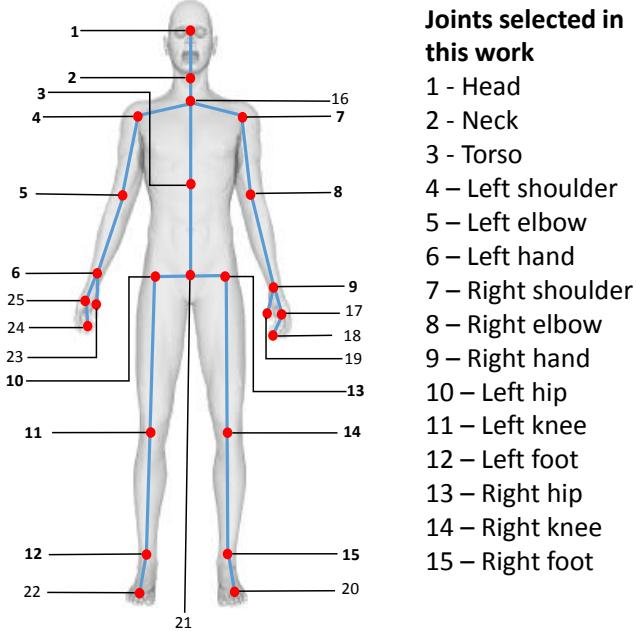
Figure 4.3: Skeleton representation of Microsoft Kinect V2 with 25 joints. 15 key joints (i.e. the highlighted joint labels) are used in this work as shown in the label definition in the figure.
