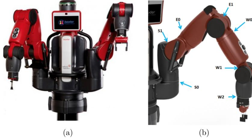
Figure 6.7: Research robot used in this work. (a) two-arm Baxter robot and (b) Baxter robot joints identification.
