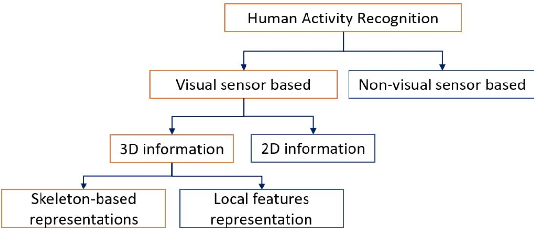
Figure 2.1: Classification of approaches widely used in human activity recognition based on the source of information.
