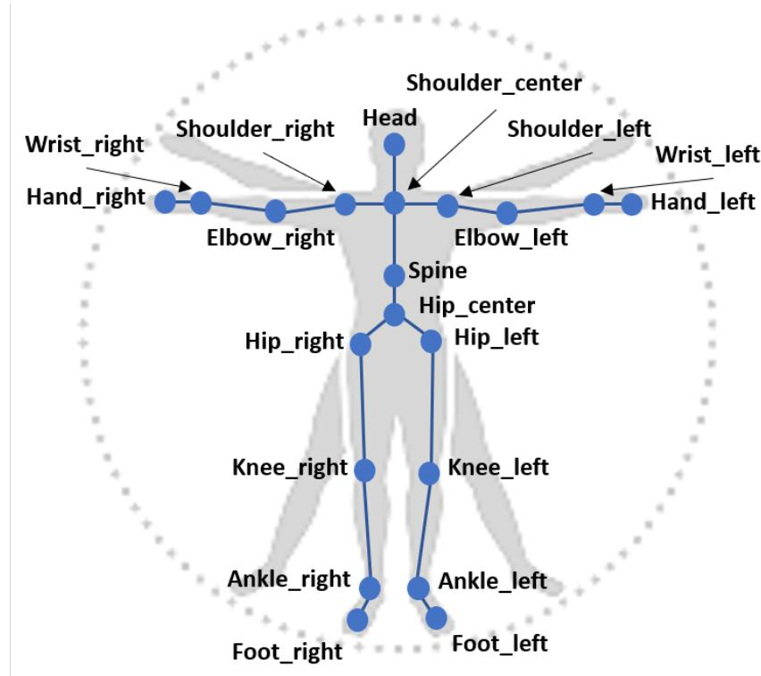
Figure 2.3: Example of skeletal body model obtained from a Microsoft Kinect device. This shows the 20 tracked joints.
