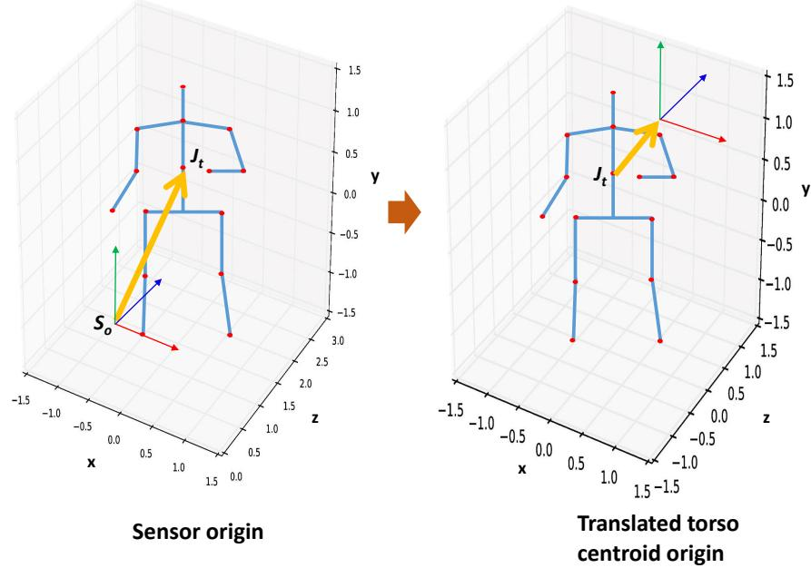
Figure 4.4: Translation of skeleton coordinate system from the sensor origin to the torso centroid origin.
