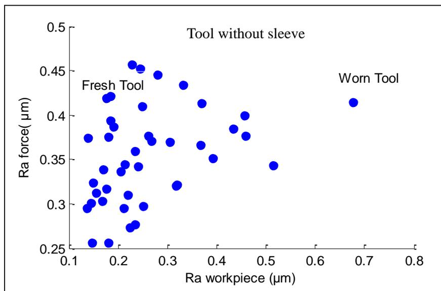
Figure 8.34: surface roughness of forces and workpiece for the tool without sleeve.
