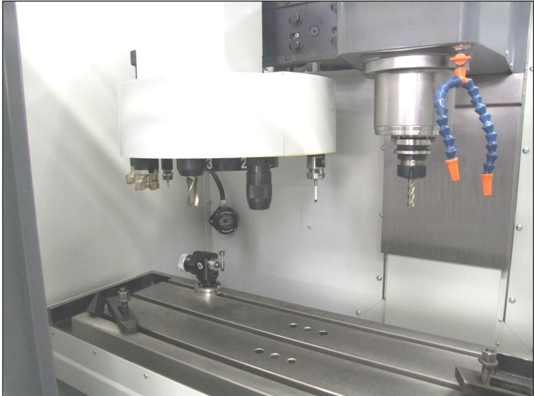
Figure 3.2: A CNC milling machine.
