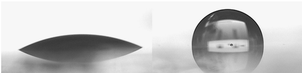
Figure 2.7: shows a sessile drop of the 1, 2 propylene glycol on SU8 layer (a) before and (b) after treatment with granger solution.
