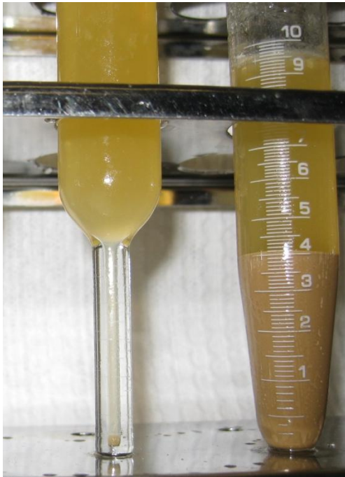
Figure 3.3: Spun volumes of centrate and the yeast cream from the disk stack process
