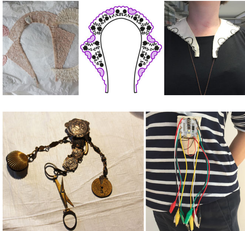
Figure 4. 'Sacrificial toiles': (top row) lace collar inspired capacitive switch using conductive ink; (bottom row) chatelaine with pin cushion, embroidery scissors and perpetual calendar, and 'lash-up' using Igloo processor board and crocodile clips, to which different sensors or outputs could be connected. Chatelaines were common in the nineteenth Century and were worn clasped at the waist; useful items were suspended on chains from the clasp. Photo: Walker and Glazzard.
