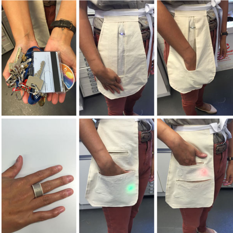
Figure 3. 'Sacrificial toiles': The pocket archetype takes on two different personalities ('generous' and 'neat') as a result of their construction, suggesting functionally and qualitatively different interaction concepts. Top row: when filled, the circuit in the generous pocket circuit is broken to light the LED. Bottom row: the conductive fabric ring completes different circuits inside the neat pocket to light different LEDs. Photo: Sarah Walker.
