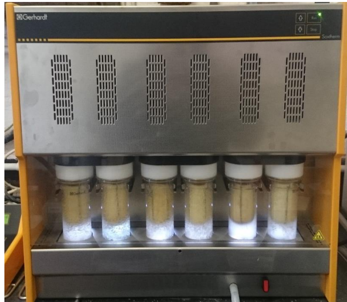
Figure 2.5. Soxtherm fat extractor (Gerhardt, UK)
