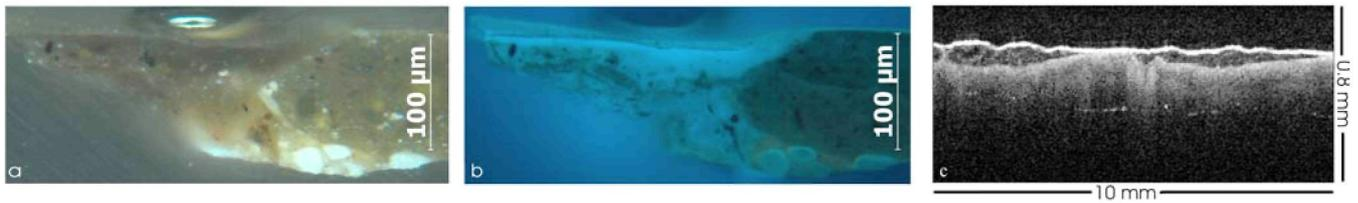
Figure 6. a) Cross-section from the foreground of the painting by Cuyp, with a crack at the left in which there are several varnish and overpaint layers, normal light; b) Cross-section in ultraviolet light; c) OCT cross-section of a similar area with multiple varnish and overpaint layers visible on the paint surface at the left of the image
