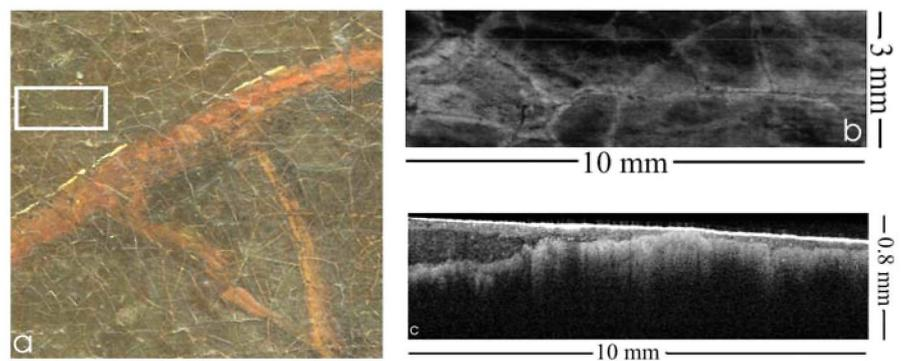
Figure 7. a) Detail of a branch in the left foreground of the painting by Cuyp. Photo © The National Gallery, London; b) *en-face* OCT image showing a loss in the paint at the left; c) OCT cross-section from the line marked on image (b), showing the loss filled with what appears to be overpaint at the left
