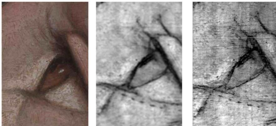
Figure 8. a) Francesco Francia, *The Virgin and Child with an Angel* (NG 3927), detail of the angel's eye. Photo © The National Gallery, London; b) Infrared image of the same region using the SIRIS camera; c) En-face OCT image at 930 nm; the size of the area on the painting is 10 by 15 mm
