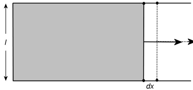
Figure 1.15: A soap film stretched over a wire frame, one end of which is movable
