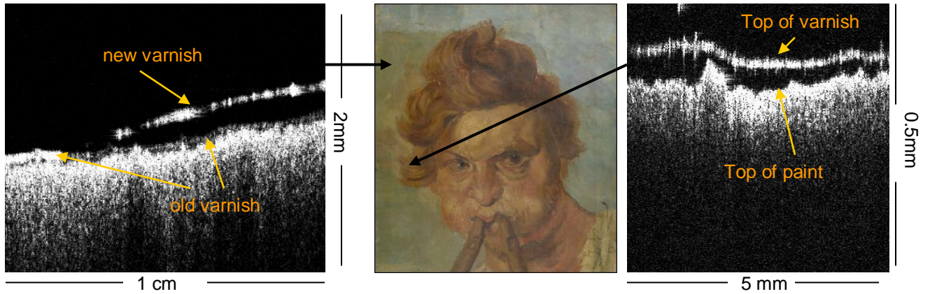
Fig 2. From left to right: 1) A cross-section image from a 1300nm OCT showing two layers of varnish above the paint layer; 2) a colour image of the painting; 3) a cross-section image from a 850nm OCT which has a higher depth resolution and X-Y resolution than the 1300nm, owing to the larger bandwidth source and higher numerical aperture used.
