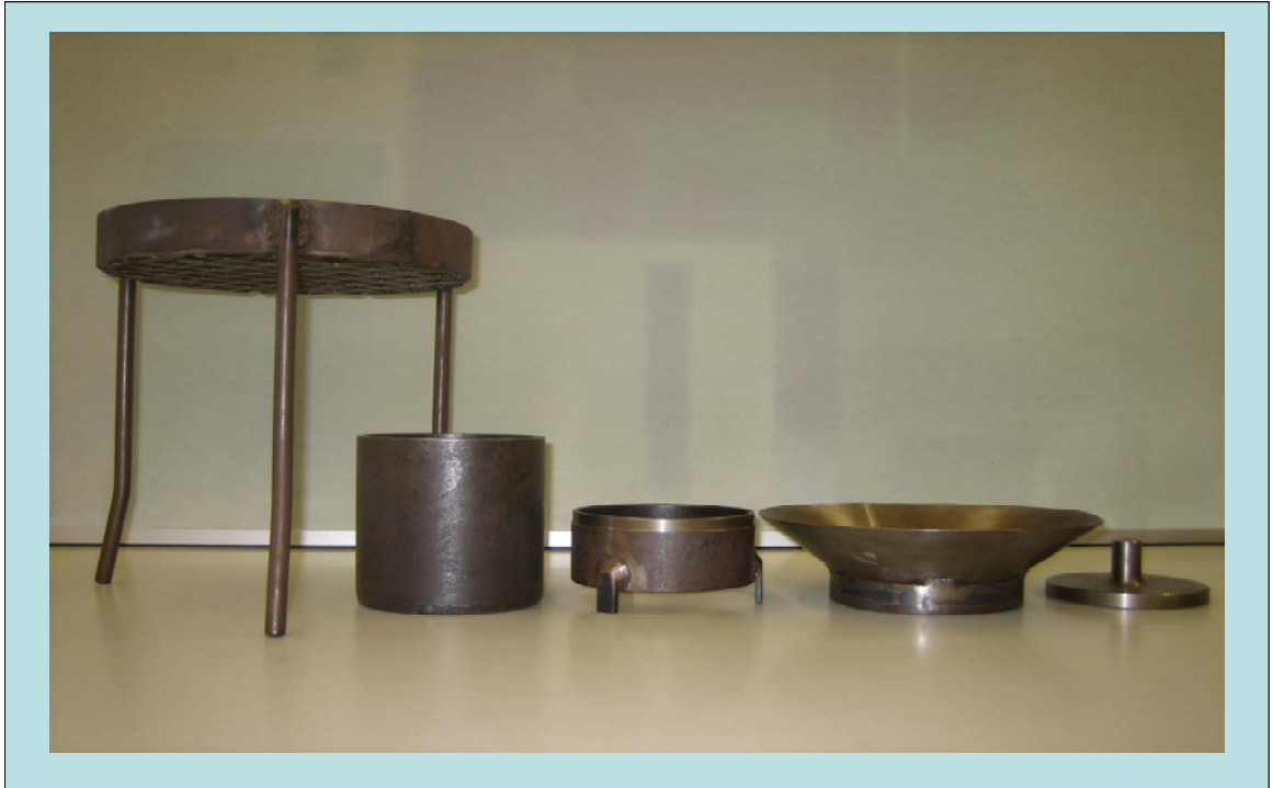
Figure 4.2.1.1: Equipment used for the determination of bulk density
