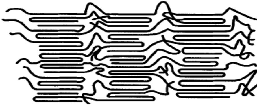
**Figure 1.5.2-5 Chain folded model of crystallisation of polymer chains**
