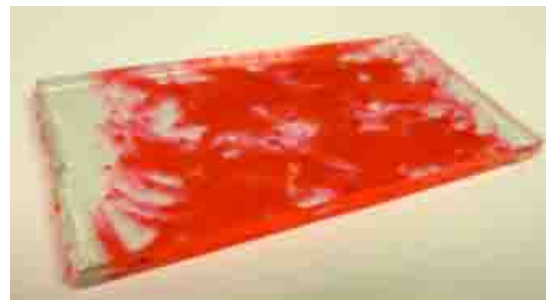
Figure 2a: EVA sheet stained with Lumogen Red 305 dye, then laminated between sheets of float glass.
