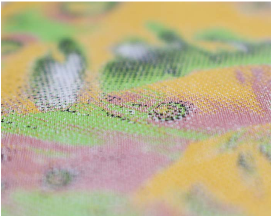
6b: Multiple colour change effect after UV exposure
