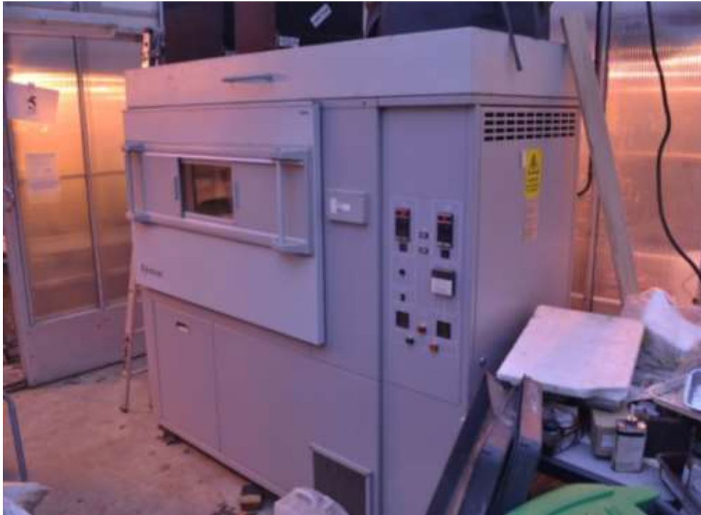
Figure 5.4 Sanyo Fitotron environmental chamber used for rearing C.vomitorea .
