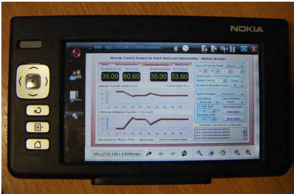
Figure B.18 Real-time monitoring interface of remote control system of solid desiccant dehumidifier for air-conditioning (Client)
