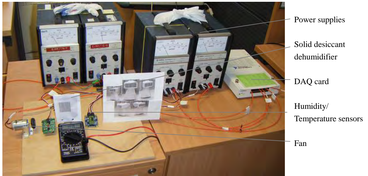
Figure 5.8 The experimental environment of the air-conditioning system with solid desiccant dehumidifier
