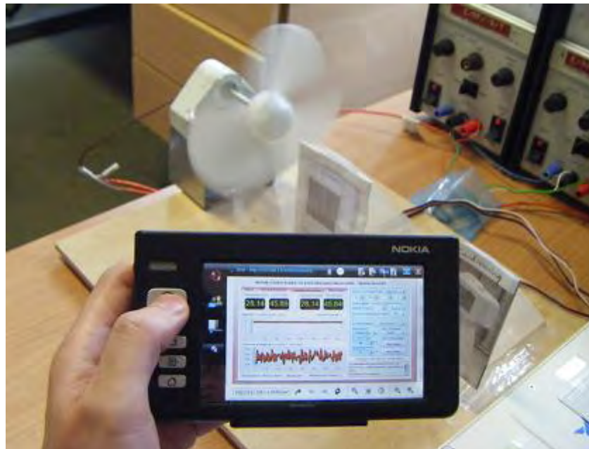
Figure 5.13 Remote control of rotation speed of the fan using the PDA and wireless Wi-Fi network
