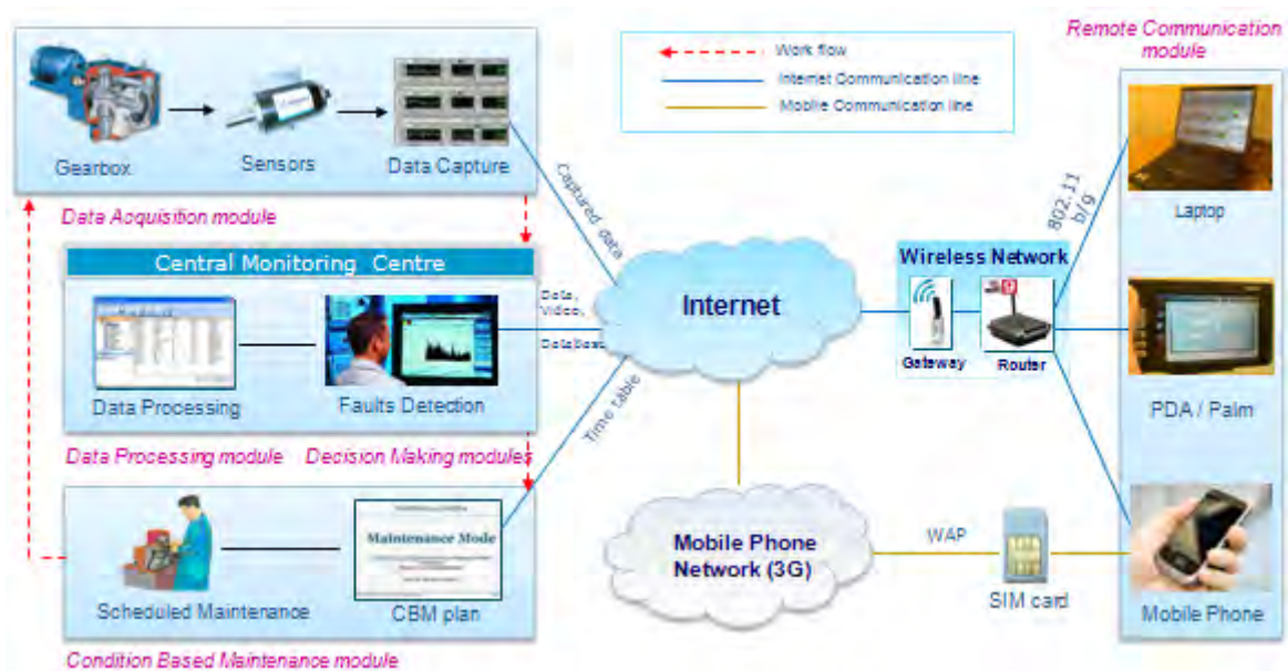
Figure 3.1 Concept model of remote real-time condition monitoring with wireless and mobile techniques
