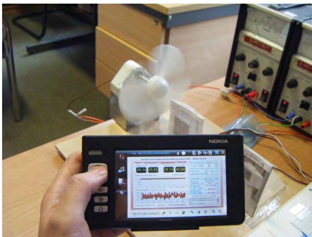
Figure B.21 Remote control interface of remote control system of solid desiccant dehumidifier for air-conditioning (Client)
