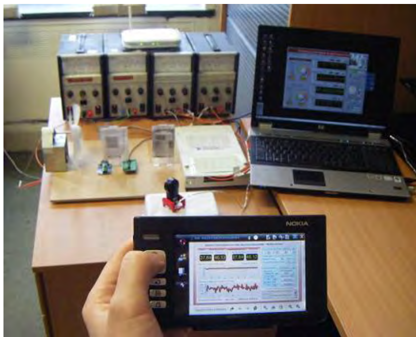
Figure 5.11 Remote access to the working condition data of solid desiccant dehumidifier used in air-conditioning system using the PDA and wireless Wi-Fi
