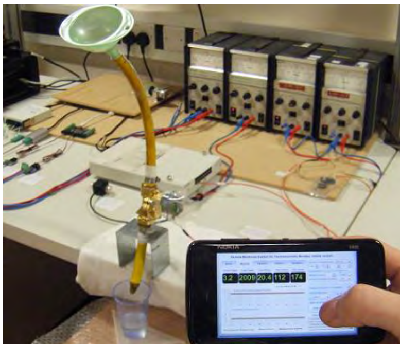
Figure 6.9 Remote control of the electric switch of the valve using Nokia mobile phone
