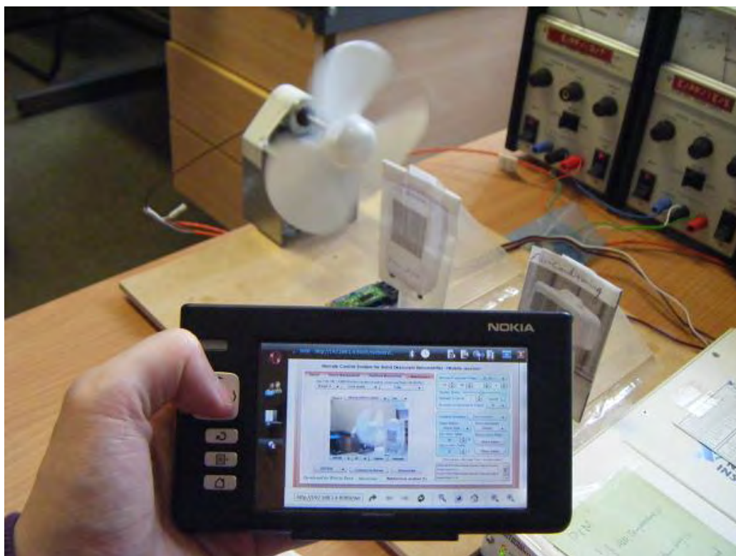
Figure B.20 remote video monitoring interface of remote control system of solid desiccant dehumidifier for air-conditioning (Client)
