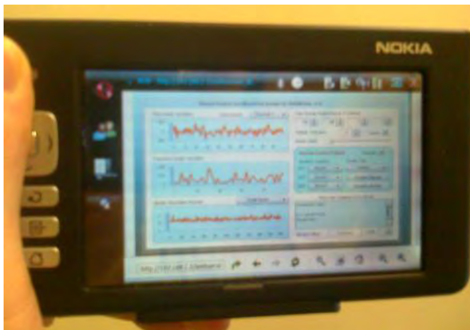
Figure 4.10 Remote access the working condition data of the server and regulate the parameters of the system using Nokia PDA via Internet and wireless Wi-Fi
