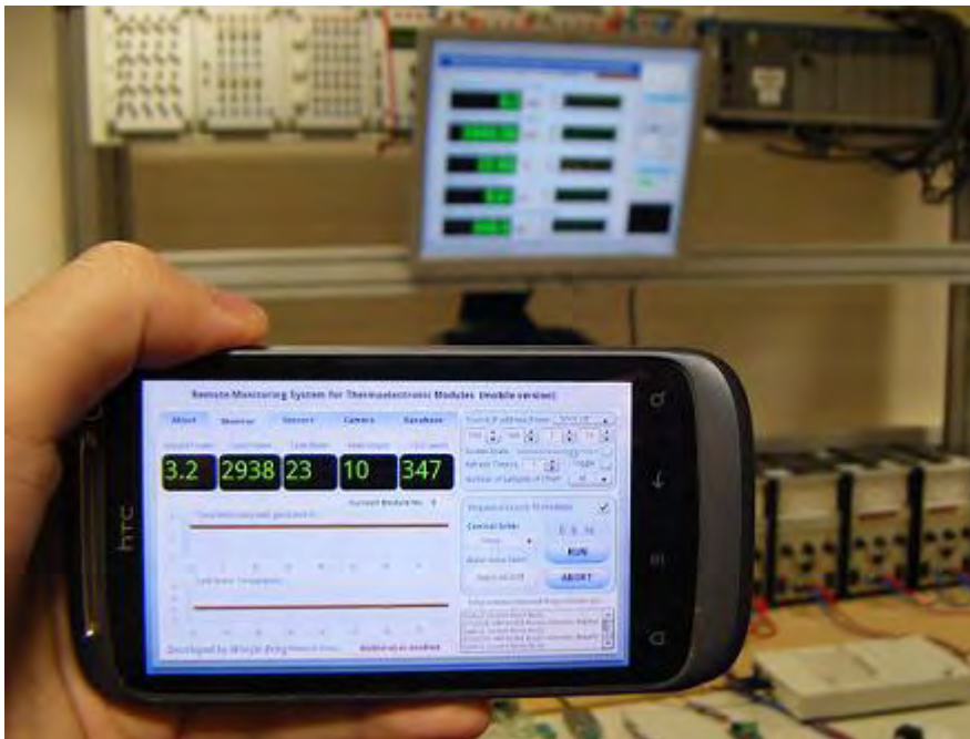
Figure 6.11 Remote acquisition of working condition data from the primary panel of the server using HTC mobile phone
