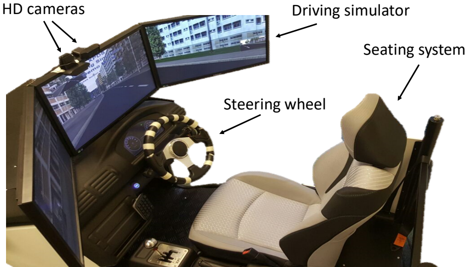
Fig. 2. Driving simulator with driver-facing cameras and high-contrast steering wheel.
