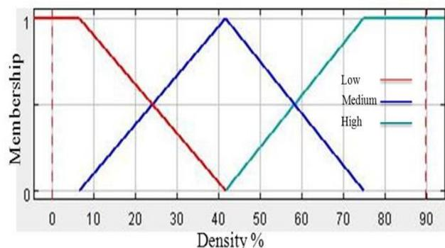
Fig. 6. Membership Functions for Longitudinal and Transverse Crack.
