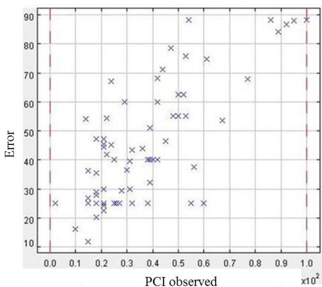
**Fig. 12.** Error of Fuzzy Pavement Classification System.
