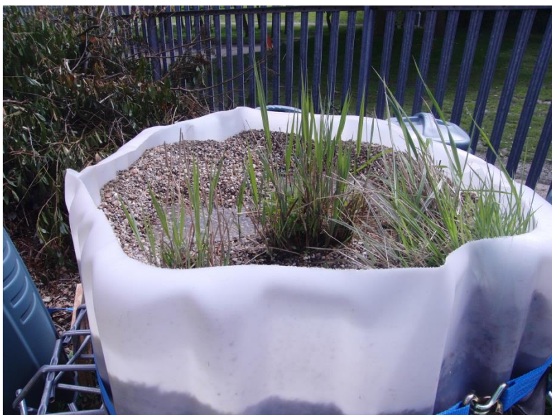
Fig. 4. An overhead photo of the prototype wetland at the Nottingham Trent University. The basis of the module was an IBC container.
