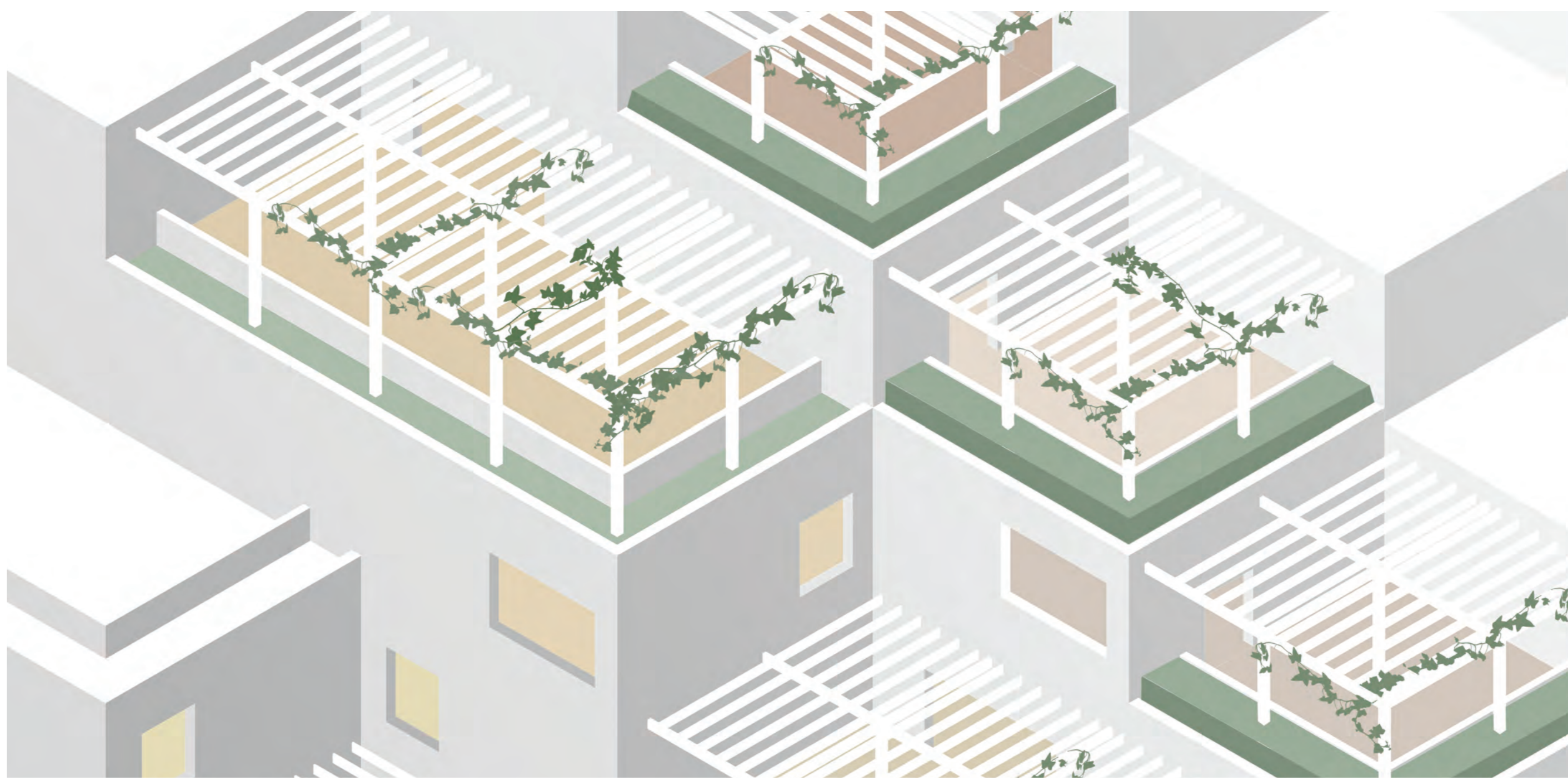
Terraces covered with pergolas provide privacy and shade from high summer sun whilst also allowing free air movement.
