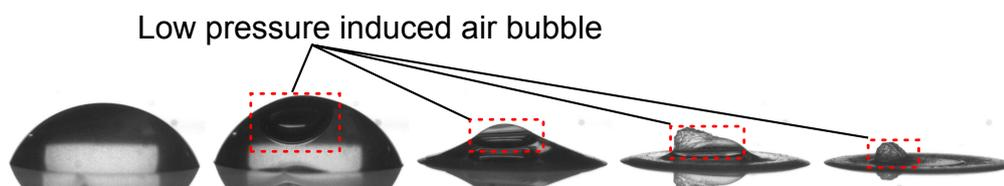
Figure 4.15: Spontaneous bubble growth at low atmospheric pressure ( $P = 100$  mbar) disrupting the droplet drying process ( $M_W = 300$  kg/mol,  $c_0 = 5\%$ ).
