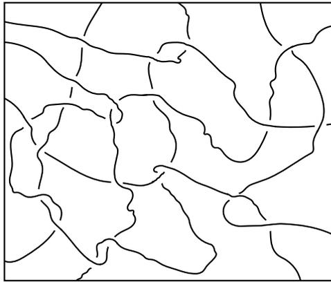
Figure 2.12: Diagram of an entangled polymer network.
