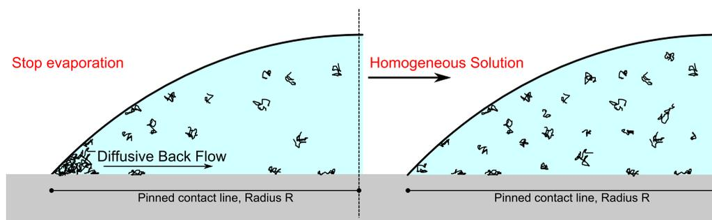
Figure 6.15: Diagram of the perfectly homogeneous system given by a droplet in which the diffusive effects outweigh the evaporative flux driven advective flow.
