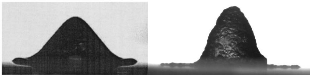
Figure 5.32: Side by side comparison of the structures that form from droplets of water dissolved: (a) Dextran,  $c_0 = 40\%$  (image taken from publication by Pauchard [124]) and (b) PEO,  $c_0 = 20\%$ .
