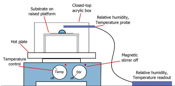
Figure 4.17: Experimental setup of temperature control with Stuart CC162 hot-plate.
