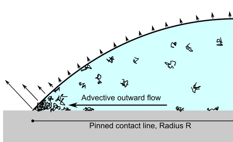
Figure 6.14: Diagram of the advective flow induced by the coffee-ring effect in a PEO droplet.
