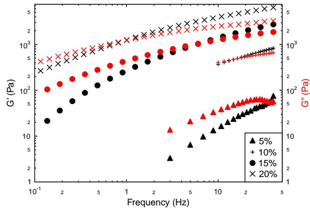
Figure 7.11: Elastic and response moduli ( $G'$  and  $G''$  respectively) plotted against frequency for PEO solutions of  $c_0 = 5, 10, 15\%$  and  $20\%$ ,  $M_W = 300$  kg/mol. Results show a crossover between viscous and elastic response at a frequency which decreases with increasing concentration.
