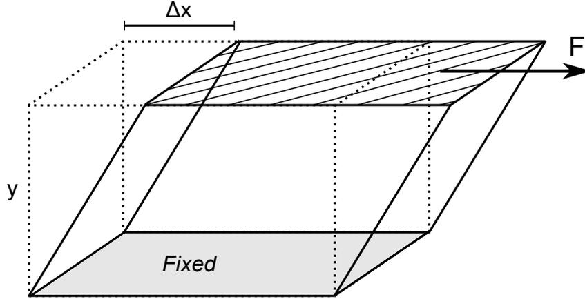
Figure 2.15: Diagram of the definition of shear deformation.
