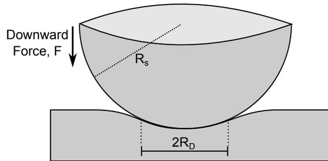
Figure 3.6: Diagram of JKR test, a method for calculating the surface tension of a solid.
