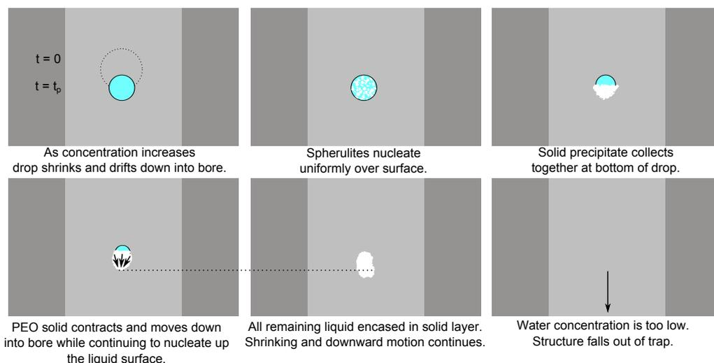
Figure 6.25: Diagram of the drying behaviour of diamagnetically levitating PEO droplets after precipitation begins. While nucleation occurs uniformly, these spherulites collect together at the base of the drop. Spherulite nucleation continues in the direction away from the precipitate up the drop surface as the solid PEO contracts and moves down into the bore. Eventually the water content of the structure is too low and it falls out of the magnetogravitational potential trap.
