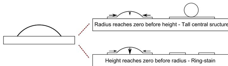
Figure 5.29: Diagram of the competing effects of precipitation driven radial receding and evaporative driven shrinking. The two outcomes show that if the radius reaches zero before the height, there will be a large central liquid region remaining once the receding stage has finished, and thus a tall central deposit, whereas if the height reaches zero first the receding phase will stop abruptly and leave behind a coffee-ring stain like deposit.
