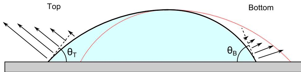
Figure 6.30: Diagram of a droplet on an incline with different contact angles at the top and bottom due to the influence of gravity. The dotted lines show the respective spherical cap shapes given by the radius of curvature at the top and bottom of the droplet.
