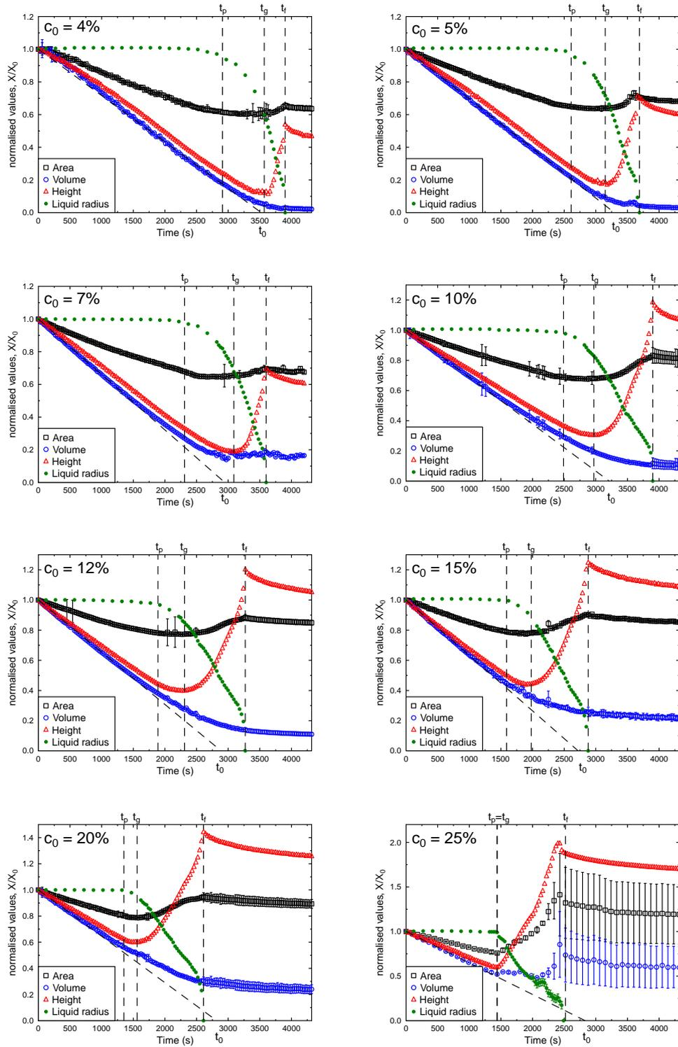
Figure 5.18: Plots of normalised surface area, volume, liquid radius and height against time for droplets of various initial concentrations.
