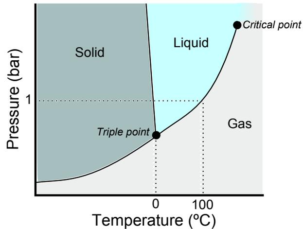
Figure 3.2: Phase diagram of water as a function of pressure and temperature
