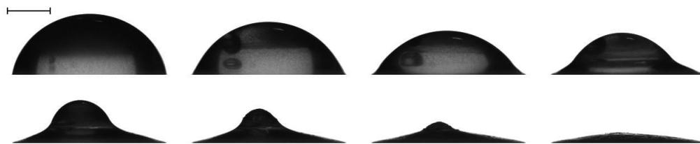
Figure 7.19: Time-lapse profile images of high molecular weight ( $M_W = 600$  kg/mol) droplet under reduced pressure ( $P = 200$  mbar) showing that the central structure formed after the surface has entirely solidified is sufficiently compressible that late stage drying reduces the structure to a flat deposit. Total time lapsed 1 hour and 10 minutes. Scale bar represents 1 mm.
