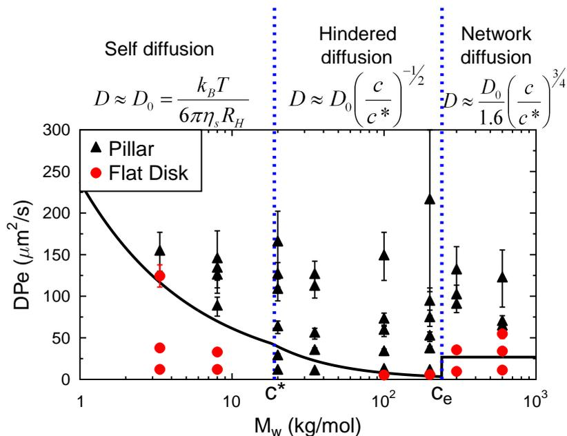
Figure 7.15: Calculated values of the  $DP_e$  for PEO solution droplets with varying evaporation rate and  $M_W$ , and initial concentration  $c_0 = 10\%$ . Differentiation is made between droplets which form pillars (black triangles) and flat deposits (red circles) and plotted against  $D$  values from the theoretical model (solid black line). Different diffusive regimes (self diffusion, hindered diffusion and cooperative diffusion) separated by dashed blue lines.
