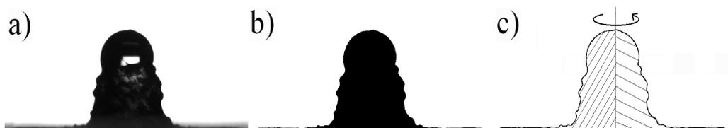
Figure 4.8: a) Profile image b) Profile image converted to binary c) Schematic of how the volume and surface area of rotation are calculated by using maximum point as the axis of rotation. Errors quantified as the difference between the rotation of the left side of the axis and the right.
