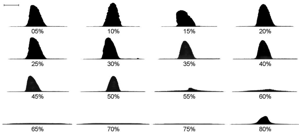
Figure 6.34: Structures formed at  $t = t_f$  from droplets of PEO-water-ethanol mixtures at ambient conditions on glass coverslips. Labels indicate initial ethanol concentration by mass. Scale bar represents 1 mm.
