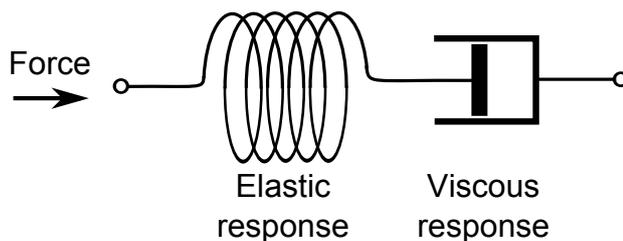
Figure 2.20: Diagram of the spring-dashpot model of the response to applied force in a Maxwellian fluid.
