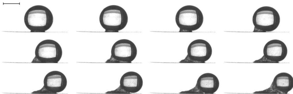
Figure 6.31: Time lapse image sequence of an elevated liquid droplet as it topples over due to structural instability, and wets the solid PEO layer. Total duration 3 minutes 40 seconds. Scale bar represents 1 mm.
