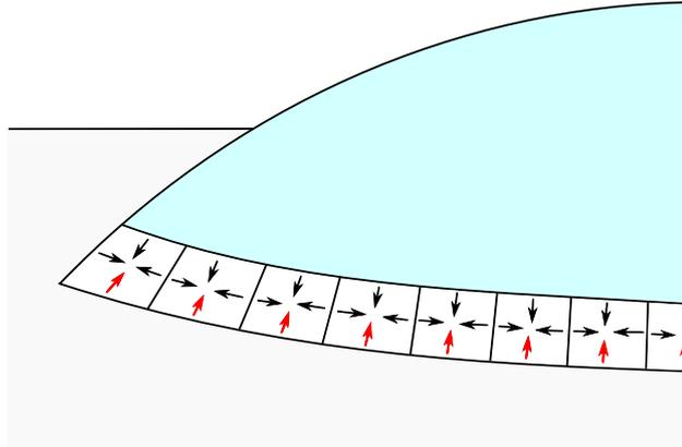
Figure 5.37: Diagram of the semi-crystalline “collar” surrounding the remaining liquid. Arrows represent the directions the spherulite boundaries must move to allow for volume loss from further evaporation from the semi-crystalline region. Red arrows represent the forbidden direction of contraction due to pinning with the substrate.
