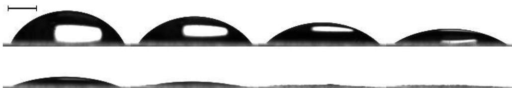
Figure 5.11: Time-lapse profile images of the drying process of a PEO droplet,  $c_0 = 3\%$ . Total duration 1hr 12mins.
