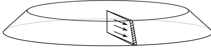
Figure 6.18: Diagram of the outward flow of polymer from the bulk of the droplet per unit length of 3 phase line.
