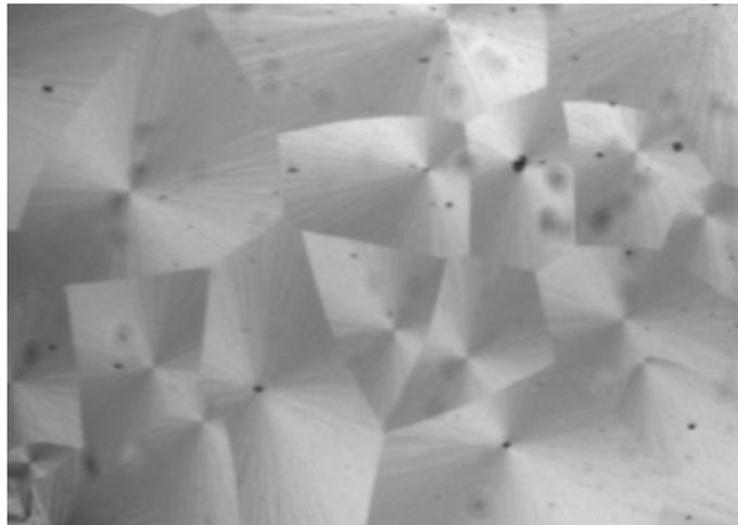
Figure 2.29: Image of spherulites captured during the late stages of drying in droplets of PEO-water solution ( $c_0 = 2\%$   $M_W = 100$  kg/mol). Nucleation occurred heterogeneously, often nucleating at dust particles.
