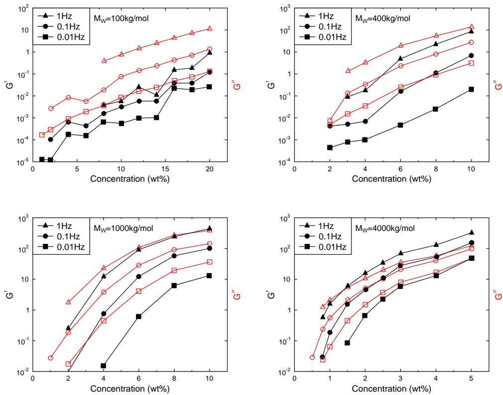
Figure 2.31: Variation of loss and storage moduli (hollow red and solid black shapes respectively) as functions of mass fraction at various oscillation frequencies for PEO solutions of  $M_w = 100, 400, 1000$  and  $4000 \text{ kg/mol}$ . Data taken from publication by Ebagninin et. al. [56]
