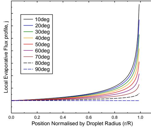
Figure 3.18: Evaporative flux profile over the surface of a sessile droplet against position  $r$  for various values of  $\theta_c$  between  $10^\circ$  and  $90^\circ$
