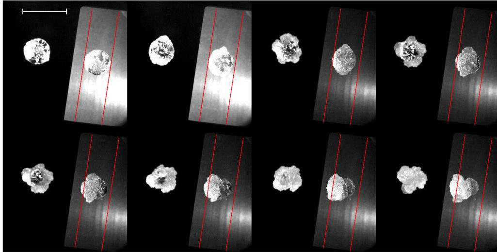
Figure 6.24: Time lapse sequence of images of a diamagnetically levitating PEO droplet after precipitation begins. Images show that precipitation occurs preferentially on one side of the droplet, which continues to contract and push itself away from the remaining liquid. Total duration 1 hour 16 minutes and 10 seconds. White bar represents 1 cm, red dotted lines added as guide to eye to show position of the solid and liquid surfaces with time relative to the droplet at  $t = t_p$ .
