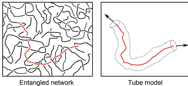
Figure 2.13: Diagram of the tube model for entangled polymer reptative diffusion.
