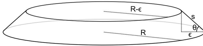
Figure 6.17: Diagram of the conical frustum over which the majority of evaporation occurs.
