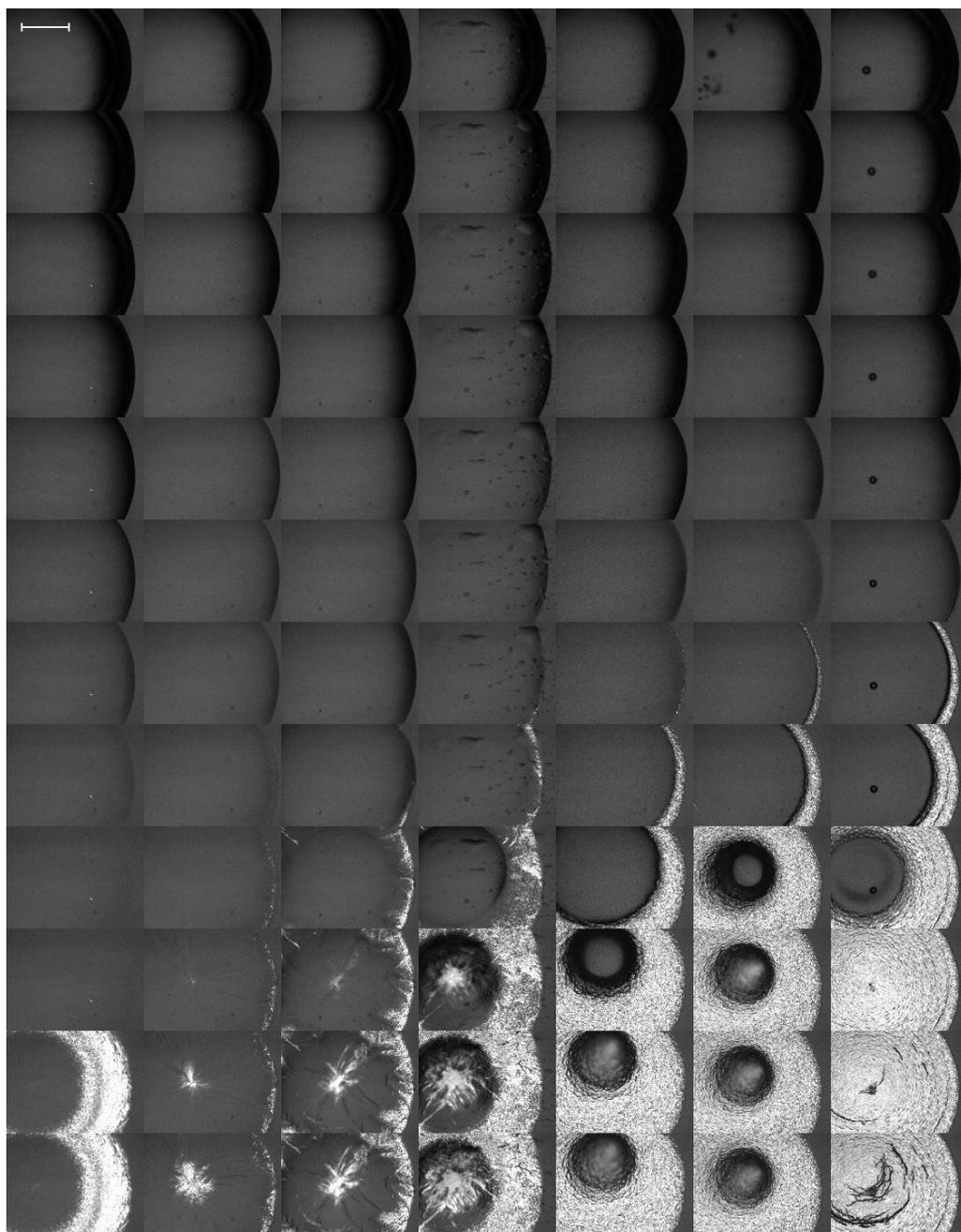
Figure 7.16: Series of vertical time-lapse images of PEO droplets as viewed under  $2\times$  magnification through cross-polarised filters. From left to right  $M_W = 3.35, 8, 2, 35, 100, 200$  and  $300$  kg/mol. Total time lapsed 4400 s. Scale bar represents 1 mm.
