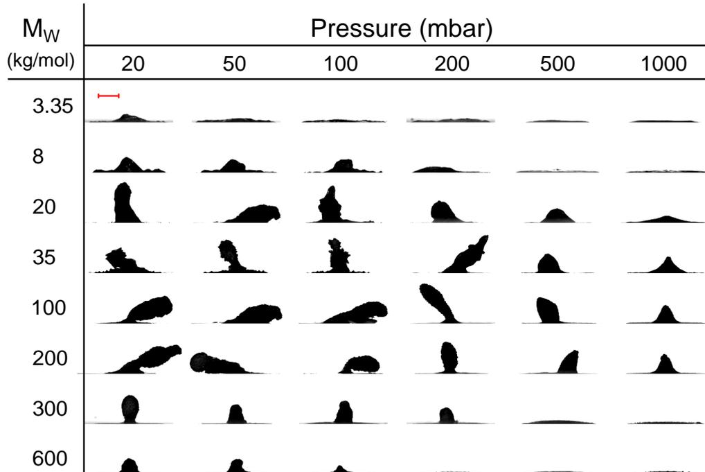
Figure 7.13: Table of fully dried droplet profile images with varying molecular weight and pressure at fixed initial concentration  $c_0 = 10\%$ . Red bar represents 1 mm.
