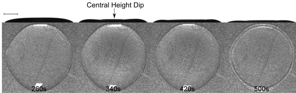
Figure 6.39: Images of a droplet with initial ethanol concentration  $c_e = 55\%$  captured from the side and above during an unusual stage in the droplet drying process in which the centre of the droplet dips to a lower height than the perimeter before precipitation begins. Scale bar represents 1 mm.
