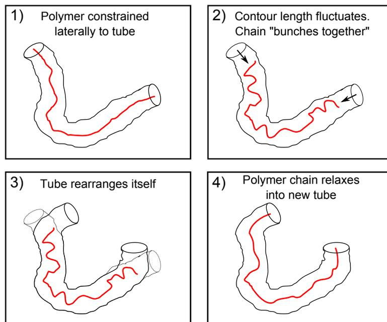
Figure 2.14: Diagram of the contour length fluctuations that lead to the discrepancies between predicted tube model and experimental values of viscosity.
