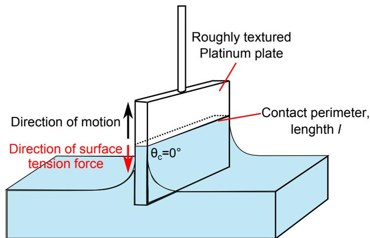
Figure 3.5: Diagram of the Wilhelmy Plate Method for calculating the surface tension of a liquid.
