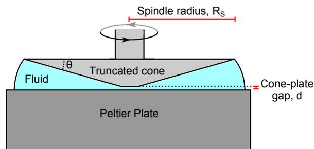
Figure 2.18: Truncated cone and plate geometry for rheology experiments
