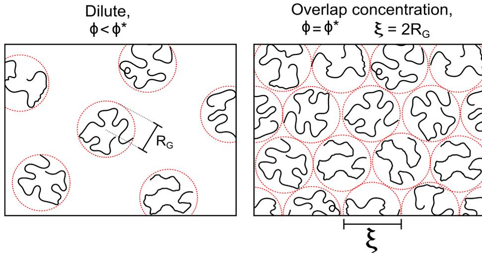
Figure 2.7: Diagram of the transition point between dilute and semi-dilute concentrations when the concentration within the pervaded volume of one polymer is equal to the concentration of the entire solution.
