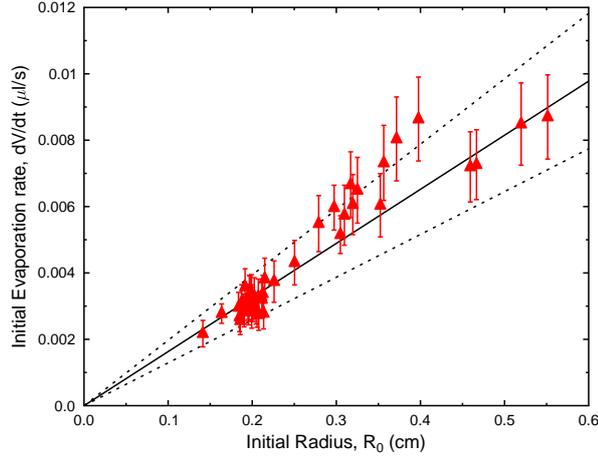
Figure 5.23: Evaporation rate for a wide range of initial concentrations and volumes, plotted against initial droplet radius  $R_0$ .
