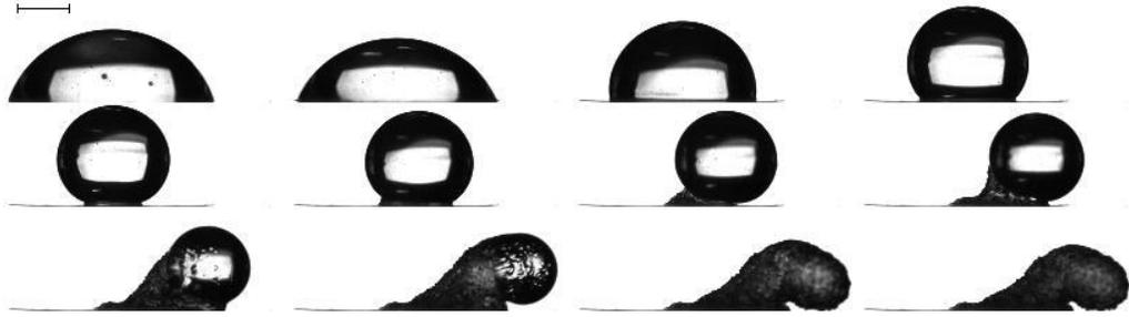
Figure 6.1: Time lapse profile images of PEO droplet,  $c_0 = 10\%$ ,  $M_W = 100$  kg/mol, at reduced atmospheric pressure of  $P = 50$  mbar. Total time lapsed 9 minutes and 10 seconds. Scale bar represents 1 mm.
