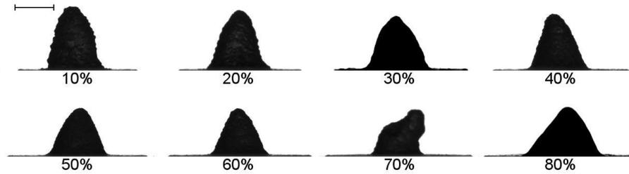
Figure 6.35: Structures formed at  $t = t_f$  from droplets of PEO-water-ethanol mixtures at ambient conditions on Granger's solution coated glass coverslips. Labels indicate initial ethanol concentration by mass. Scale bar represents 1 mm.
