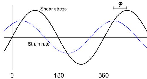
Figure 2.19: Plot of shear stress and shear rate against oscillation angle for a fixed angular frequency. The strain rate is out of phase with shear stress by angle  $\varphi$ .
