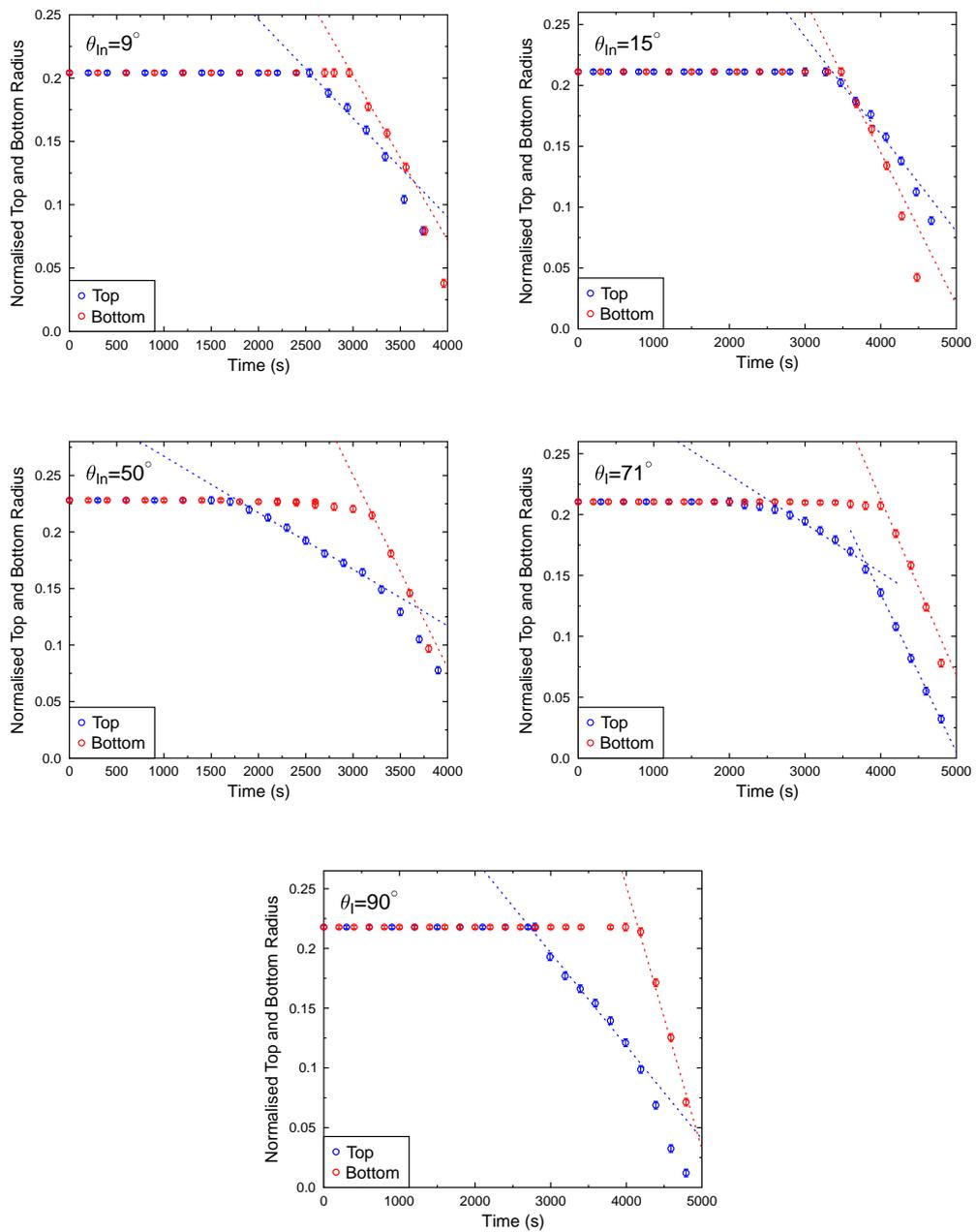
Figure 6.28: Series of radius versus time plots at angles of inclination  $\theta_{in} = 9, 15, 50, 71$  and  $90^\circ$ . The blue and red plots are measurements of the top and bottom radius as the distance between the centre of the initial droplet and the top and bottom 3-phase lines.
