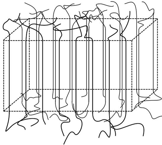
Figure 2.27: Diagram of a chain folded lamella, the basic unit of the semi-crystalline polymer structure. Individual polymer contour lengths are much longer than the thickness of the ordered region.
