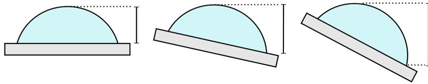
Figure 6.29: Diagram of the effective height increasing with the angle of inclination. When this effective height increases above the capillary length ( $\lambda_c \approx 2$  mm for water), assuming high hysteresis, the droplet bulges down in the direction of gravity.
