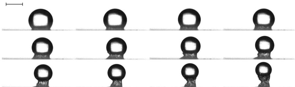
Figure 6.32: Time-lapse sequence of images illustrating the contraction of the thin supporting solid structure leading to height increase of the liquid phase. Total duration 3 minutes 51 seconds. Scale bar represents 1 mm.
