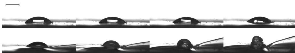
Figure 5.39: Time-lapse profile images of a PEO droplet drying on a thin sheet of PDMS. Once precipitation begins (in the fourth image), the substrate is pulled upwards by forces induced by the combination of a contracting PEO collar and a high pinning forces between the droplet and the substrate. Scale bar represents 2 mm.
