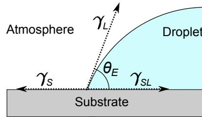
Figure 3.4: Diagram of the directional forces acting at the three interfaces between solid, liquid and air in a sessile droplet. Young's relation is found by equating the solid-air interfacial tension  $\gamma_S$  with the sum of the solid-liquid interfacial tension  $\gamma_{SL}$  and the x-component of the liquid-air interfacial tension  $\gamma_L \cos \theta_E$ .
