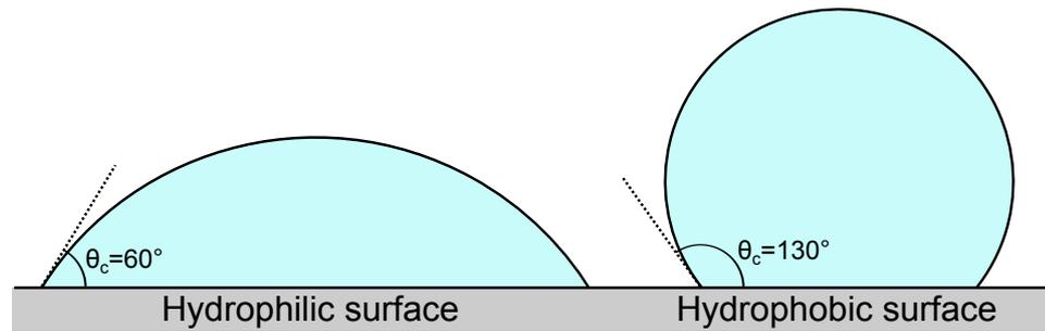
Figure 3.8: Diagram of side by side comparison of two equal volume water droplets on hydrophilic and hydrophobic surfaces.
