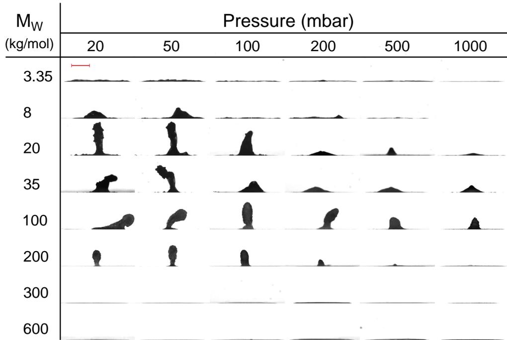
Figure 7.12: Table of fully dried droplet profile images with varying molecular weight and pressure at fixed initial concentration  $c_0 = 5\%$ . Red bar represents 1 mm.
