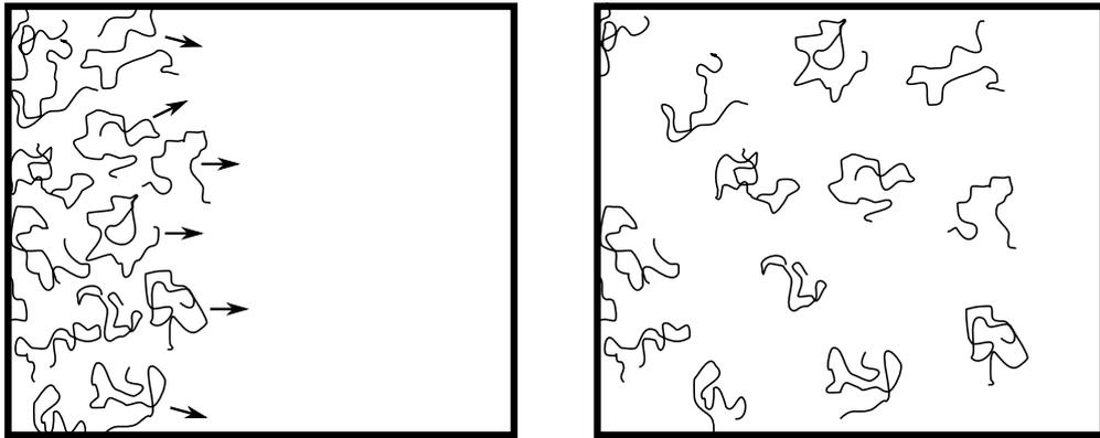
Figure 2.10: Diagram of the effect of cooperative diffusion. A concentration gradient leads to a greater degree of freedom in the direction of lowest concentration. Random motion leads to polymers cooperatively diffusing down a concentration gradient.
