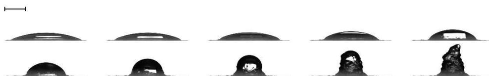
Figure 5.9: Time-lapse profile images of drying droplet during stage three - boot-strap building. Total duration 13.5 min. Scale bar represents 1 mm.
