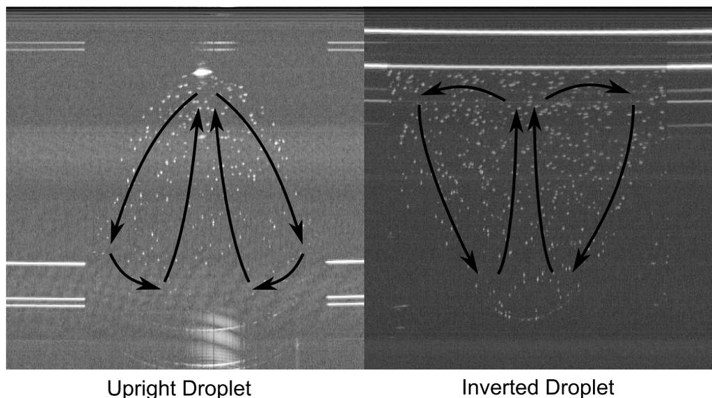
Figure 7.8: Comparison of direction of convection currents observed via OCT in an upright and inverted PEO droplet ( $c_0 = 5\%$ ,  $M_W = 20$  kg/mol). Findings show that when the droplet is inverted, the direction of flow remains downward at the droplet-air interface and upward in the centre, suggesting density changes at the surface (or buoyancy) is the driving force behind convection.
