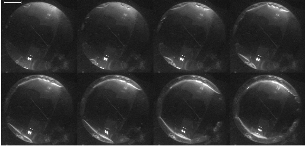
Figure 5.30: Time-lapse sequence of images showing that occasionally precipitation begins non-uniformly around the perimeter of the droplet. Scale bar represents 1 mm.
