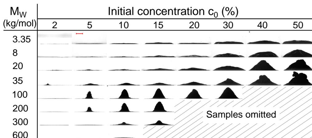
Figure 7.3: Table of fully dried droplet profile images with varying  $M_W$  and  $c_0$  in atmospheric conditions  $T = 22 \pm 2^\circ\text{C}$  and  $RH = 35 \pm 5\%$ . Samples in the lower right region were omitted due to difficulties of depositing  $10 \mu\text{l}$  droplets of such high viscosity liquids. Red bar represents 1 mm.
