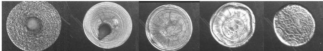
Figure 6.11: Fully dried images of droplets dried in an oven at temperatures (from left to right)  $T = 21, 30, 40, 50$  and  $60^\circ\text{C}$  captured from above.  $c_0 = 10\%$ .
