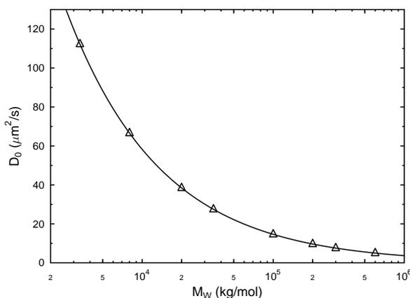
Figure 7.4: Plot of  $D_0$ , the self diffusion coefficient at very low concentrations calculated using equation 7.1, against polymer molecular weight. Triangles represent values of  $M_W$  used in these experiments.
