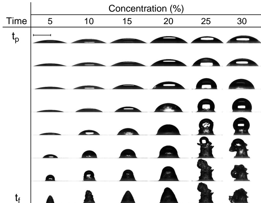
Figure 5.17: Six vertical time-lapse droplet image sequences captured during the pseudo-dewetting and boot-strap building stages. From left to right, initial concentration  $c_0 = 5, 10, 15, 20, 25$  and  $30\%$ . From top to bottom is the time axis, with total time taken equal to the difference between the precipitation time and the time at which surface crystallisation stops ( $t = t_f - t_p$ ). Scale bar represents 2 mm.
