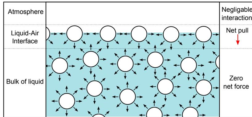
Figure 3.3: Diagram of the intermolecular cohesive forces acting between liquid molecules in both the bulk and at the surface of the liquid, resulting in a net inward pull at the interface, or surface tension.
