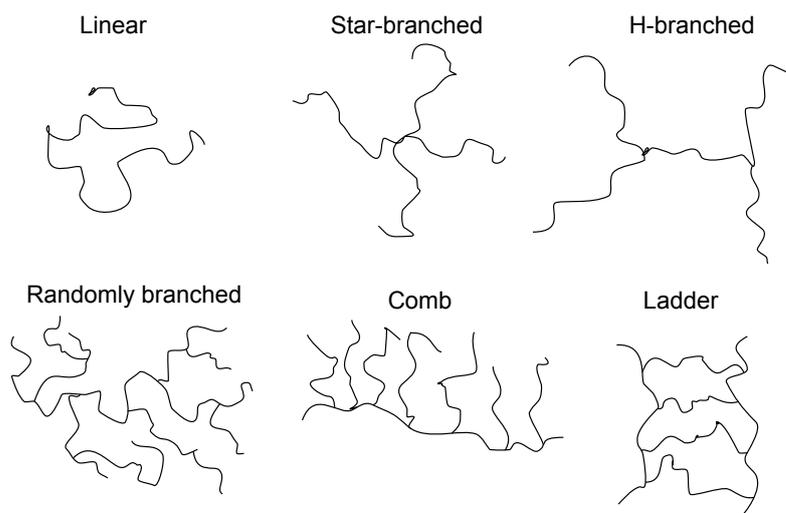
Figure 2.1: Diagram of several examples of polymer architecture including: linear, star-branched, H-branched, randomly branched, comb and ladder structures.
