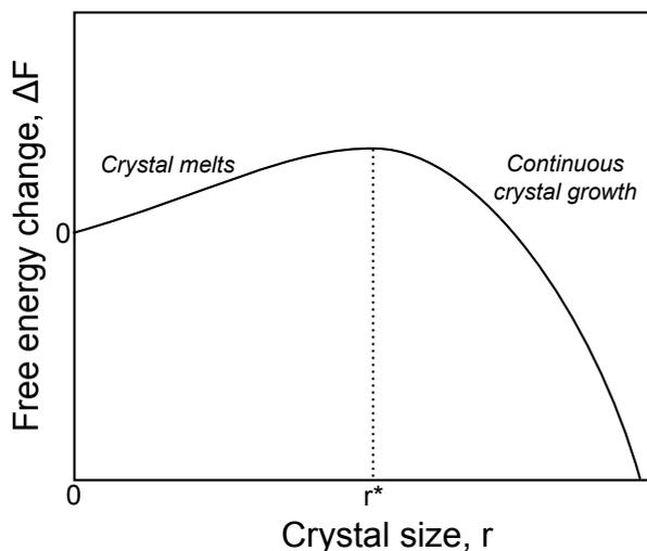
Figure 2.28: Schematic plot of the change in free energy as a function of crystal size.
