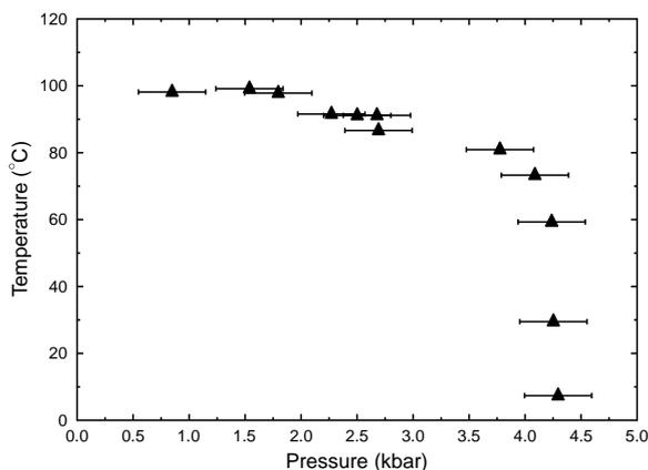
Figure 2.24: Plot of lower critical solution temperature (LCST) values for PEO solution ( $c_0=0.001\text{g/g}$   $M_W = 270 \text{ kg/mol}$ ) as a function of pressure and temperature. Data published by Cook et. al. [46].
