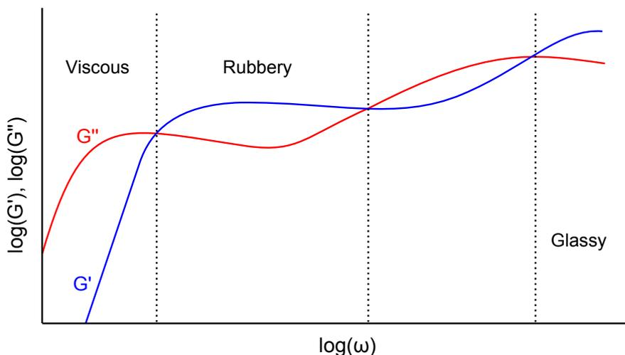
Figure 2.22: Plot of typical  $G'$  and  $G''$  curves as a function of oscillation frequency for a polymeric fluid.
