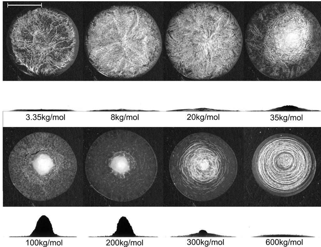
Figure 7.2: Fully dried deposits as viewed from the side and above with varying PEO molecular weight. Concentration fixed at  $c_0 = 10\%$ . Scale bar represents 1 mm.
