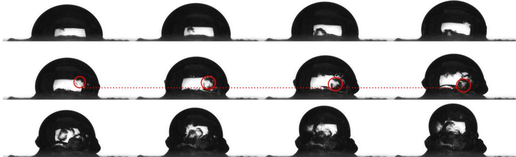
Figure 5.35: Sequence of images during the bootstrap building stage of  $c_0 = 25\%$  droplet. The semi-crystalline region advances up the surface of the remaining liquid. Red circles highlight a single spherulite that initially grows until it comes into contact with another spherulite, and then appears to move down toward the substrate.
