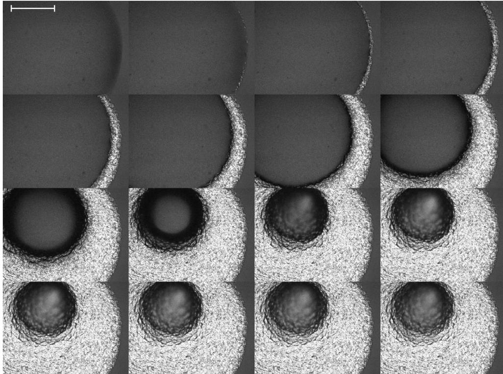
Figure 5.3:  $2\times$  magnification images of 10% PEO droplet, captured from underneath through cross-polarized filters. Time step between images 2.5 min. Scale bar represents 1 mm.
