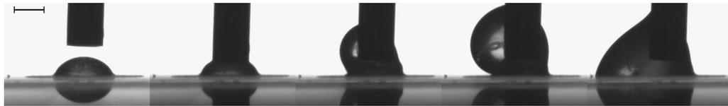
Figure 6.26: Series of profile images captured during the inflation of a PEO droplet with further PEO solution during the pseudo-dewetting stage. The influx of liquid leads to a build up in the centre with a fixed base radius. This continues until the volume is sufficiently large that it spills over the spherulite collar and wets the thin layer of deposited solid PEO. Scale bar represents 1 mm.
