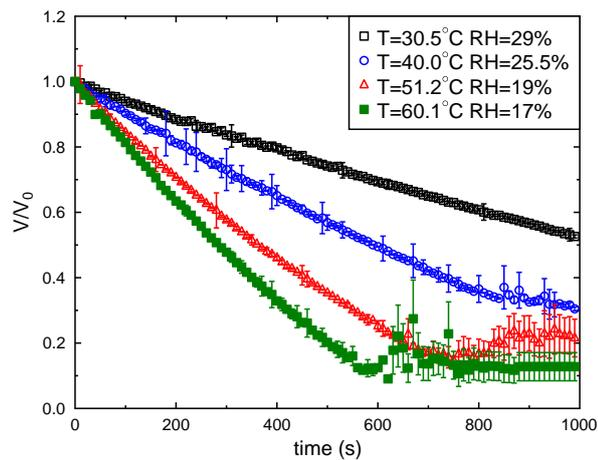
Figure 6.12: Normalised volume curves for droplets evaporating at various atmospheric temperatures. This plot shows that evaporation rate increases with temperature.
