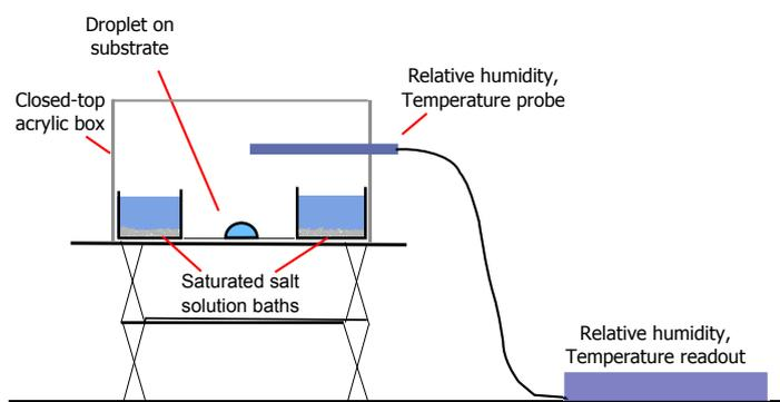
Figure 4.16: Experimental setup of relative humidity control.
