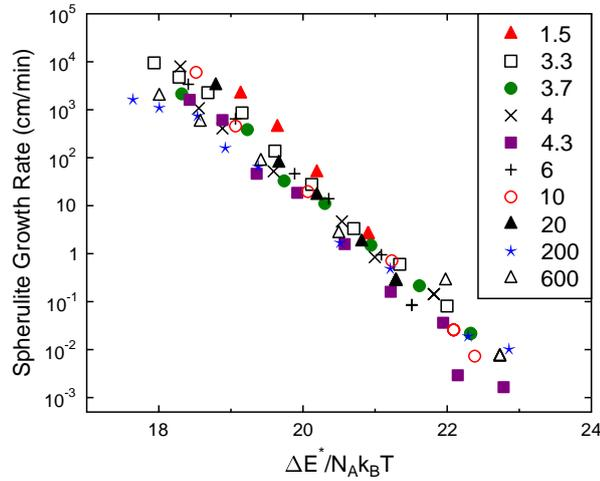
Figure 2.32: PEO Spherulite growth rate as a function of  $\Delta E^*/N_A k_B T$  (where  $\Delta E^*$  is the free energy of the nucleation of a spherulite with critical size  $r^*$  and  $N_A$  is avagadros number) for various values of molecular weight, labeled in the key in units of kg/mol. Data taken from publication by Beech et. al. [57].
