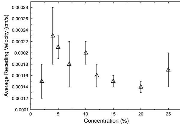
Figure 5.19: Plot of the average receding speed during stages 2 and 3 as a function of initial concentration.
