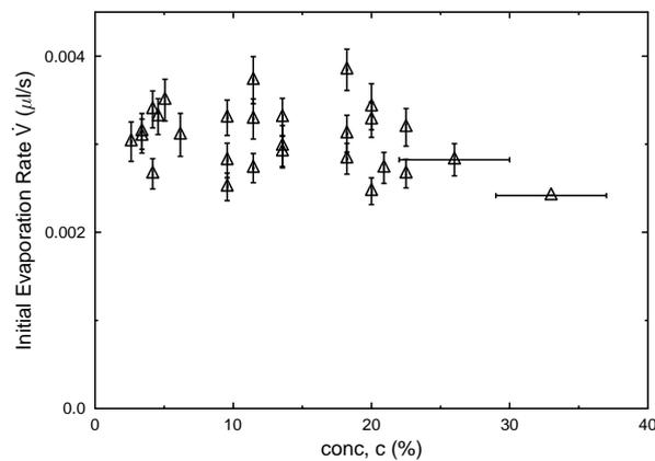
Figure 5.21: Plot of initial evaporation rate  $\dot{V}$  against initial droplet concentration.
