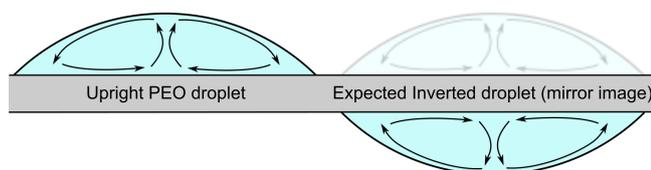
Figure 7.7: Diagram of the expected effect of inverting the droplet on the direction of convection currents.
