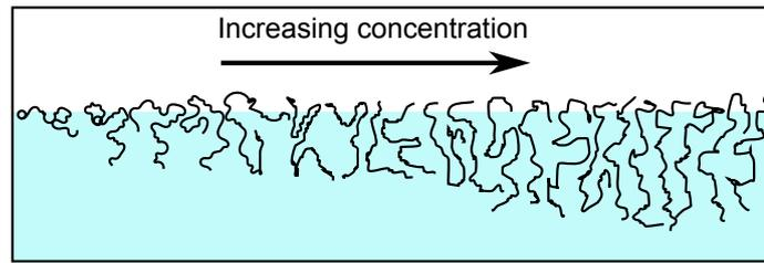
Figure 3.13: Diagram of arrangement of PEO chains at air-water interface with increasing concentration [82]. Single chains preferentially lie along the surface at low concentrations. They begin to bunch up and dangle into the liquid as concentration is increased.
