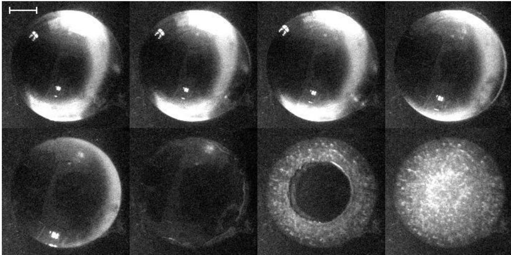
Figure 5.12: Time-lapse images of the drying process of a PEO droplet,  $c_0 = 3\%$ , as viewed from above. Total duration 1hr 12mins.
