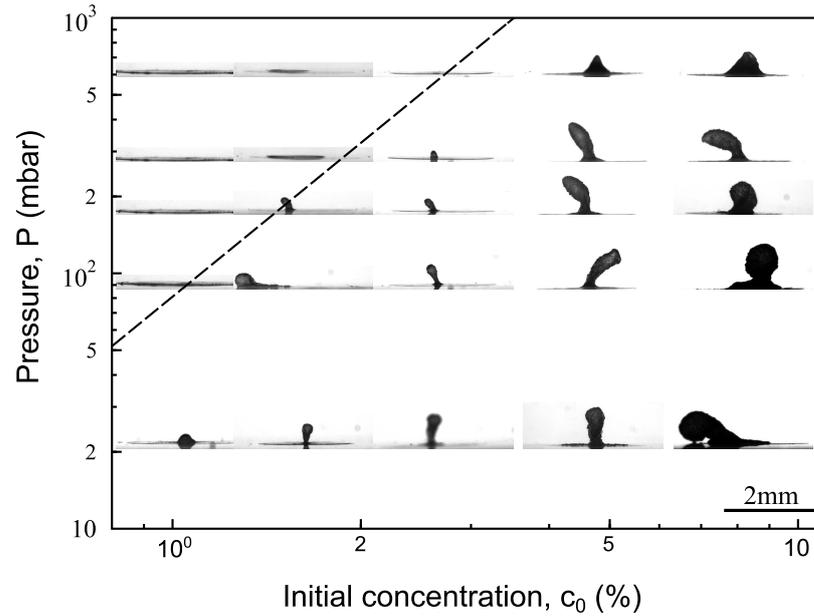
Figure 6.5: The shape of the solid deposit at the end of stage 3 plotted as a function of both initial droplet concentration  $c_0$  and reduced pressure  $P$  on log axes. The dashed line is a guide to the eye dividing pillars (below) from flat deposits (above) and has the form  $P \propto c_0^2$ .
