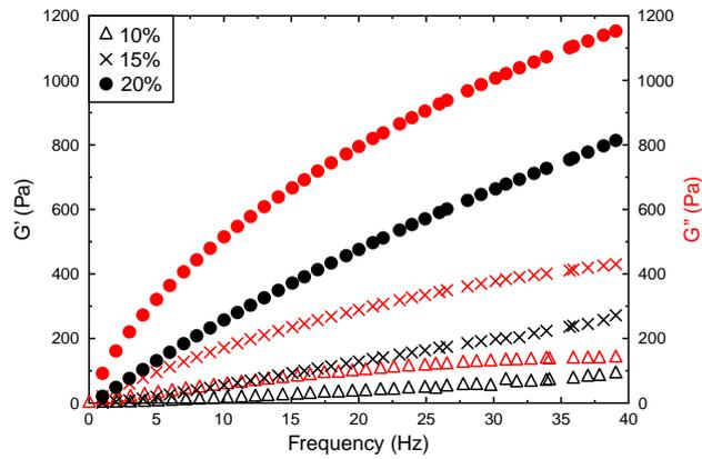
Figure 7.10: Elastic and response moduli ( $G'$  and  $G''$  respectively) plotted against frequency for PEO solutions of  $c_0 = 10, 15$  and  $20\%$ ,  $M_W = 200$  kg/mol. The viscous response is dominant in the concentration and frequency range observed.
