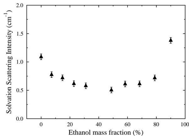
Figure 6.40: Scattering intensity versus ethanol mass fraction with PEO concentration  $c_0 = 10\%$ . This data was originally published by Hammouda [40] for ethanol-water mixtures at  $T = 50^\circ\text{C}$  and PEO volume fraction  $\phi = 4\%$ , which has been rescaled for total ethanol mass fractions of water-ethanol-PEO solutions to match the data in this work.
