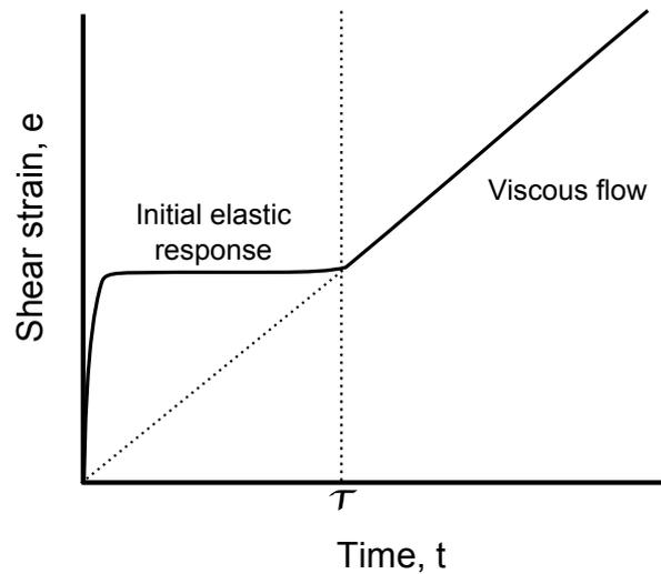
Figure 2.17: Schematic plot of the shear strain at a fixed shear stress as a function of time in a viscoelastic fluid.
