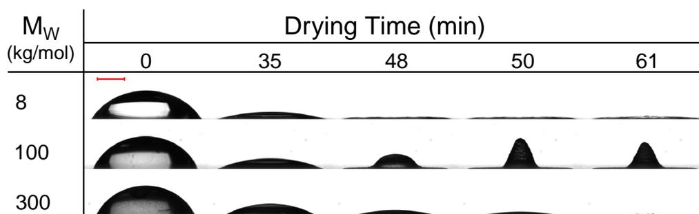
Figure 7.1: Time-lapse profile images of droplets drying at ambient conditions at 0, 35, 48, 50 and 61 minutes.  $M_W = 8, 100$  and  $300$  kg/mol in top middle and bottom rows respectively. Red scale bar represents 1 mm.
