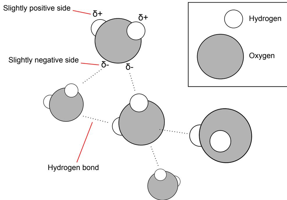
Figure 3.1: Random arrangement of liquid water molecules. The more strongly electronegative Oxygen causes an uneven charge distribution around the molecule, or polarity. The attraction this polarity causes between water molecules is known as hydrogen bonding.
