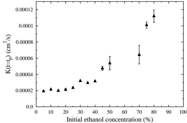
Figure 6.38: Plot of  $K$  (the proportionality between evaporation rate  $\dot{V}$  and droplet radius  $R$ ) immediately prior to PEO precipitation against initial droplet ethanol concentration.
