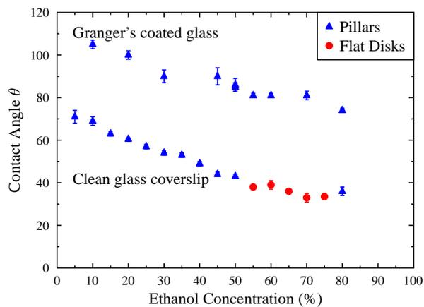
Figure 6.36: Plots of initial contact angle against ethanol concentration on both clean and Granger's solution coated glass coverslips.
