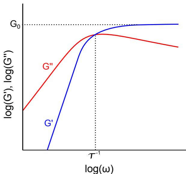
Figure 2.21: Representative plot of storage and loss modulus as a function of oscillation frequency for a Maxwellian viscoelastic fluid.
