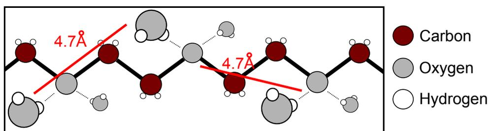
Figure 2.23: Schematic of a simplified view of the likely arrangement of a PEO chain dissolved in water. The distance between water molecules and the next nearest neighbour is exactly equal to the inter-oxygen distance along the PEO backbone.
