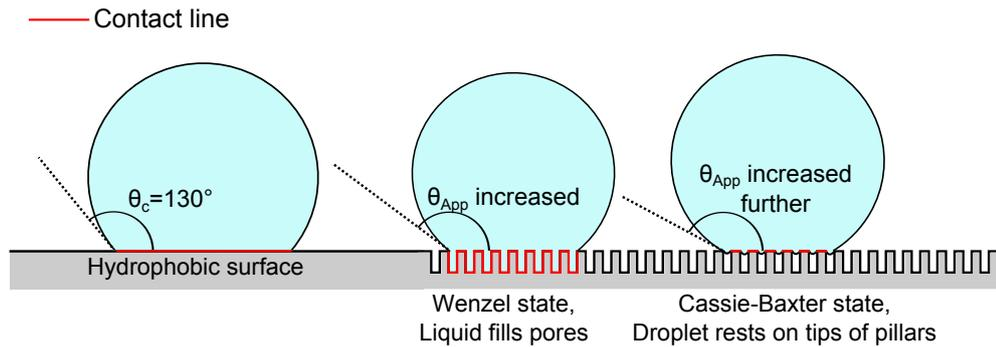
Figure 3.10: Diagram of comparison between wetting on a hydrophobic smooth surface and the effect of Wenzel and Cassie-Baxter state on the contact angle of a water droplet
