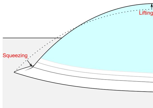
Figure 5.38: Diagram of contracting collar induced receding of the liquid phase.
