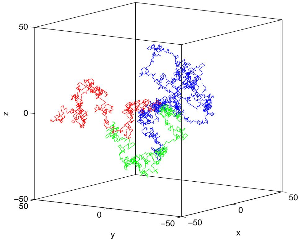
Figure 2.4: Plot of three different random walks of 750 steps (each step length equal to one unit in space) in three dimensions.
