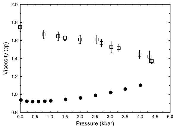
Figure 2.25: Viscosity measurements with increased pressure for water [47] (filled circles) and PEO solution,  $M_W = 270$  kg/mol  $c_0 = 0.1\%$  (hollow squares). Data published by Cook et. al. [46].
