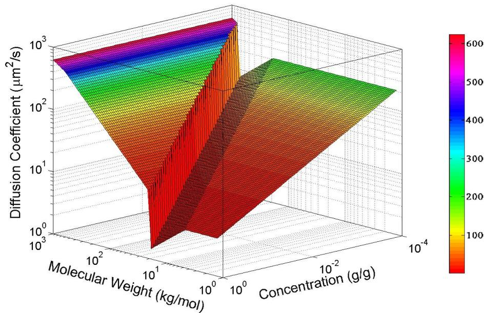
Figure 7.14: Theoretical 3D plot of the diffusion coefficient of PEO in solution with varying concentration and molecular weight. Dip shows predicted high Péclet number region.
