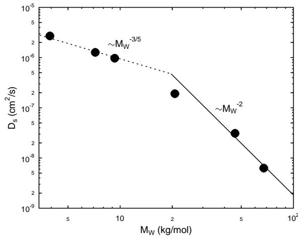
Figure 2.11: Plot of self diffusion coefficient as a function of molecular weight at constant concentration. Solid lines show predicted dilute and semi-dilute self diffusive behaviour. Data points agree with these predictions but show a gradual, rather than a sudden, transition between the two regimes. Data published by Zettl et. al. [18].
