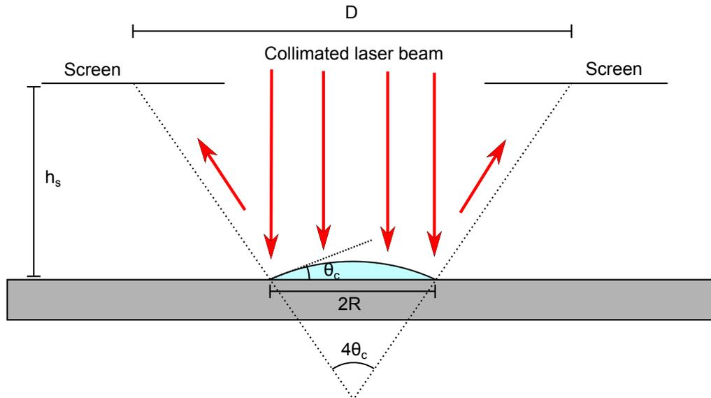
Figure 3.7: Diagram of optical reflectometry method for calculating the contact angle of a deposited droplet, for droplets with  $\theta_c < 45^\circ$
