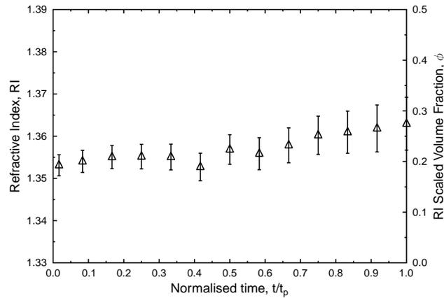
Figure 6.19: Average refractive index across the central vertical region of a PEO droplet ( $c_0 = 5\%$ ,  $M_W = 100$  kg/mol) plotted against time normalised by the precipitation time,  $t/t_p$ .
