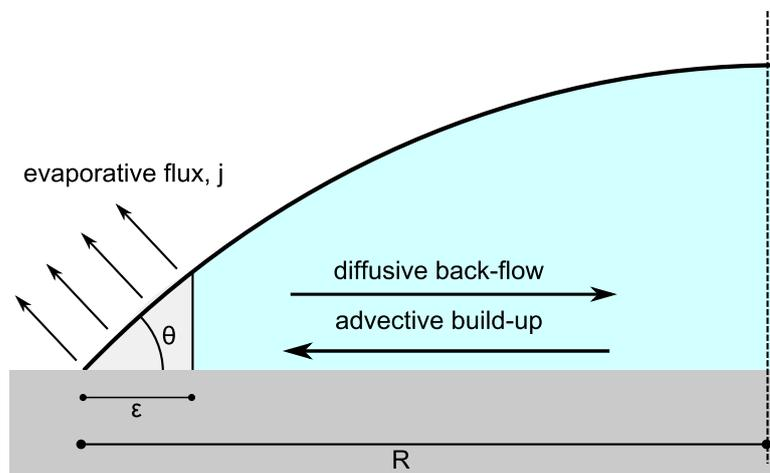
Figure 6.16: Diagram of the first major assumption of the Péclet number characterisation: the vast majority of evaporation occurs in a narrow triangular wedge close to the 3-phase line.
