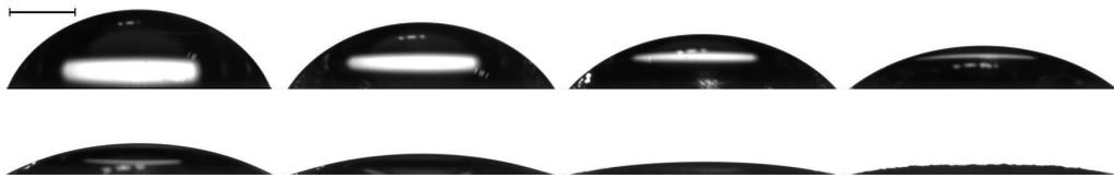
Figure 6.8: Time-lapse profile images of  $c_0 = 10\%$  droplet drying at high relative humidity  $RH = 81 \pm 2\%$ . Total time lapsed 2 hours and 3 minutes. Scale bar represents 1 mm.
