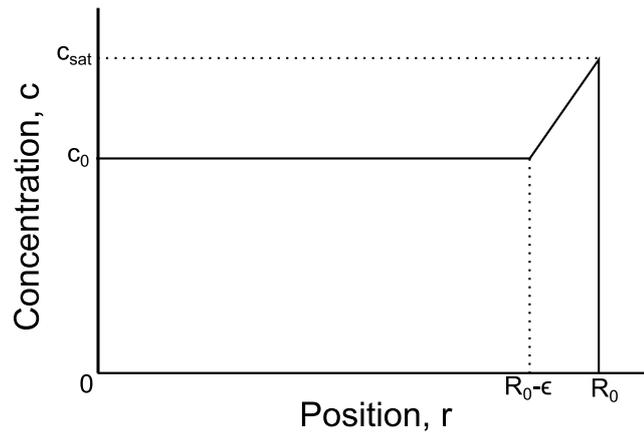
Figure 6.20: Schematic plot of the assumed concentration profile at  $t = t_p$ .
