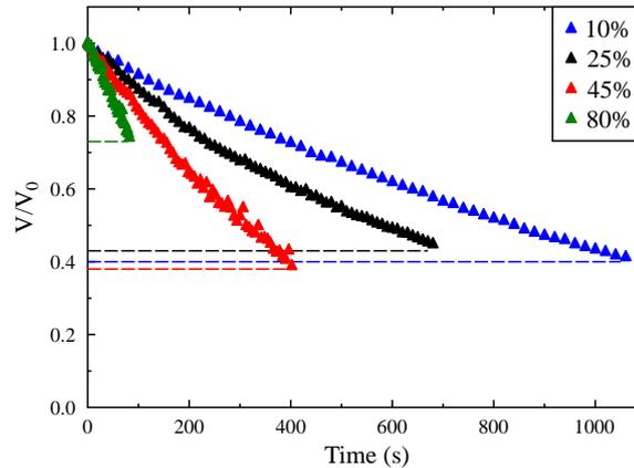
Figure 6.37: Plots of  $V/V_0$  against time for various initial ethanol concentrations on clean glass substrates. Dashed lines mark the fractional volume when precipitation begins and remains fairly constant for  $c_e = 10, 25$  and  $45\%$ , but is significantly higher at  $c_e = 80\%$ .
