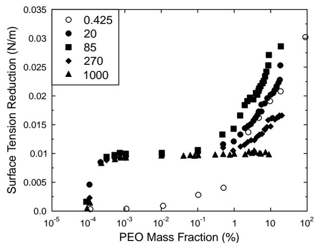
Figure 3.14: Plot of the change in surface tension against PEO concentration for a range of molecular weight. Different molecular weights distinguished by key in units of kg/mol. Plotted data taken from publication by Cao [83].
