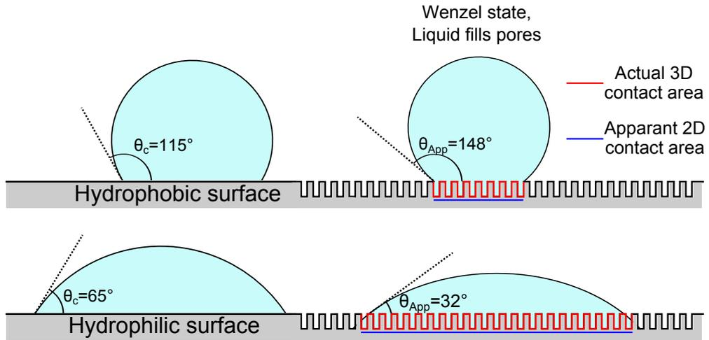
Figure 3.9: Diagram of Wenzel state wetting. The liquid fills the pores, and the apparent contact angle is either increased if the original smooth surface was hydrophobic, or decreased if it was hydrophilic. Calculated apparent angles for the case when  $A_{3\text{D}} = 2A_{2\text{D}}$
