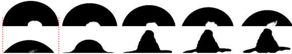
Figure 5.26: Profile images of a  $c_0 = 10\%$ ,  $V_0 = 10 \mu\text{l}$  droplet on a Cytop coated substrate. Red dotted lines added to aid clarity to the comparison between initial radius and droplet radius immediately prior to precipitation. At late stages of drying the droplet peels itself away from the substrate. Images courtesy of Manon Granjard from the University of Edinburgh.
