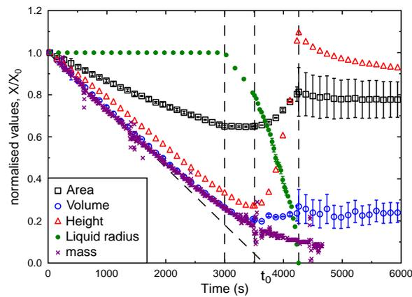
Figure 5.4: Plot of normalised surface area, volume, mass, liquid radius and height against time for a single PEO droplet, initial concentration  $c_0 = 10\%$  calculated from droplet profiles. Vertical dashed lines separate time into four stages: pinned drying; pseudo-dewetting; boot-strap building; and late stage contraction. Diagonal dashed line represents volume and mass trajectory from initial drying rate and crosses horizontal axis at  $t = t_0$ .
